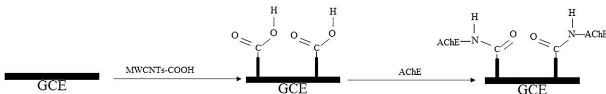
Fig. 1. Assembling AChE on glassy carbon electrode: ultrasonicated MWCNTs were adsorbed and layered on polished surface of GCE following doping of AChE through amide bond formation.
