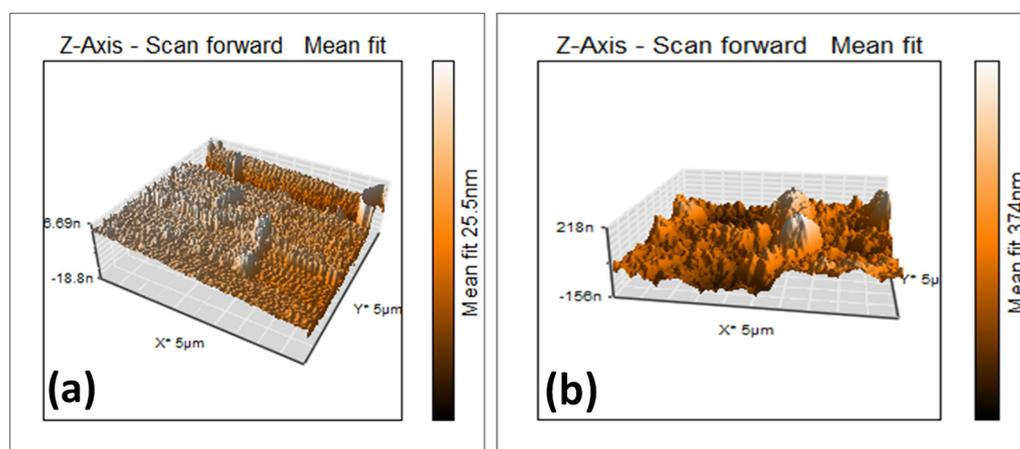
Fig. 3. AFM pictures of different electrode surfaces: (a) bare polished glassy carbon electrode; (b) MWCNTs modified and AChE doped glassy carbon electrode (AChE/MWCNTs/GCE).
