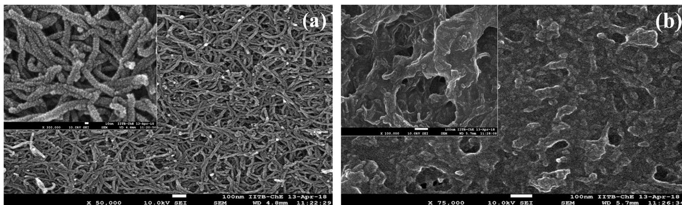
Fig. 2. SEM Images of modified electrode surfaces: (a) MWCNTs adsorbed (MWCNTs/GCE); (b) AChE doped on MWCNTs (AChE/MWCNTs/GCE).
