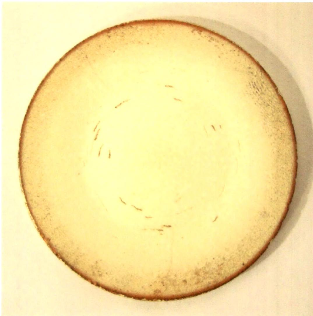
**Figure 5.5: i-ZnO target having diameter of 50 mm ( $\pm$  1 mm) prepared using method of grouting and sintering.**
