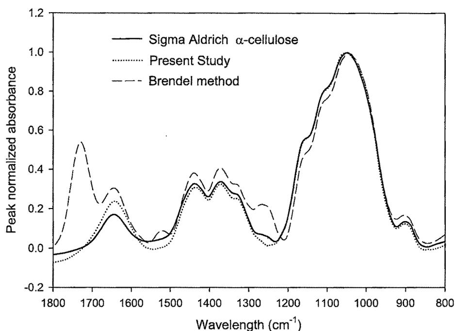
**Fig.2.10.** Representative FTIR spectra of  $\alpha$ -cellulose extracted using present method, Brendel et al., (2000)'s method and commercial available  $\alpha$ -cellulose of Sigma Aldrich.
