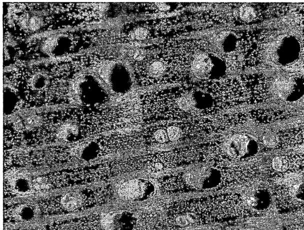
**Fig.2.8.** Ring porous vesicle structure observed in the teak samples.
