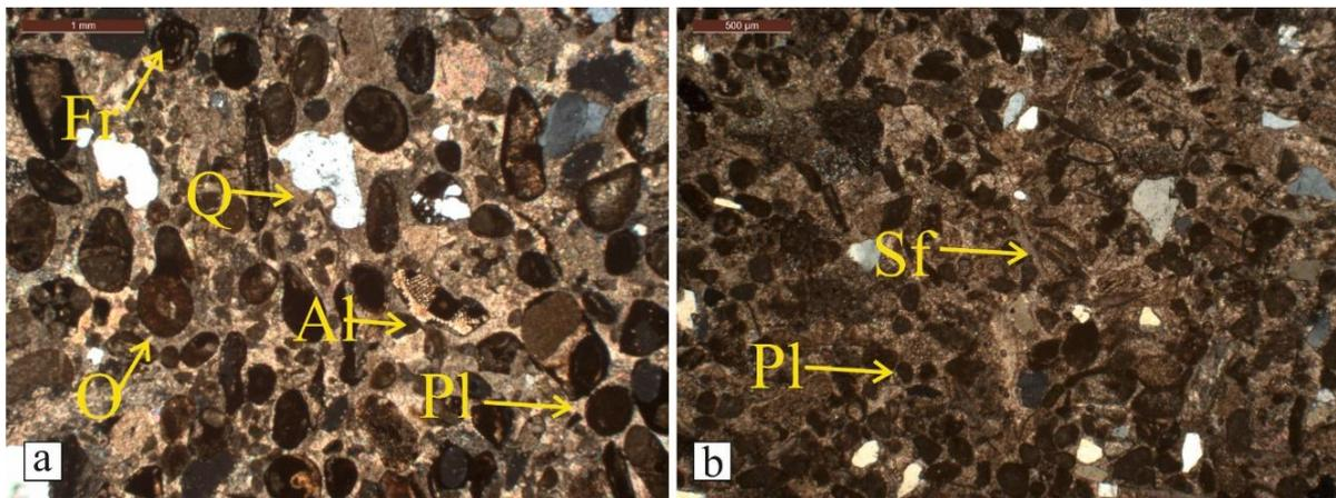
Plate 4.4(a) Photomicrographs of pelloidal wackestone-packstone containing algae (Aa), forams (Fr), onchoids (O), quartz (Q) and reworked pellets (Pl). (b) Photomicrographs of pelloidal wackestone-packstone containing abundant Pellets (Pl) and shell fragments (Sf) and algae.
