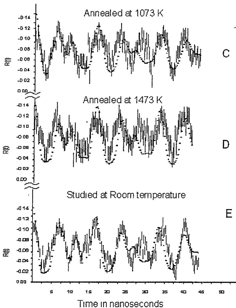
Fig 2 TDPAC spectra of sample at annealing temperatures 1073 K ( C ), 1473 K (D) Spectra E is studied at Room temperature
