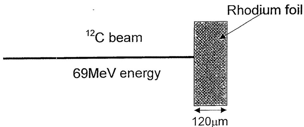
Fig 5.1 Block Diagram of Experimental set up
