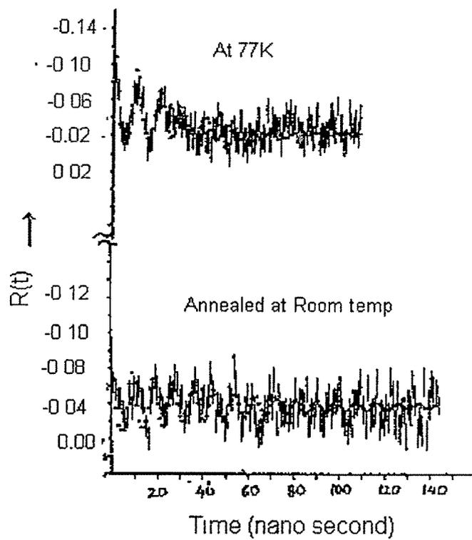
Fig 3 TDPAC Spectra of sample at 77K and 300K
