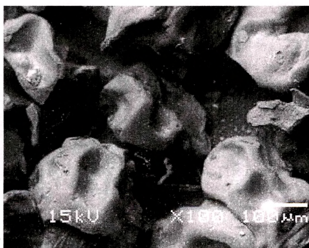
Figure 9.7: The scanning electron micrograph of dried alginate beads at 100X magnification.
