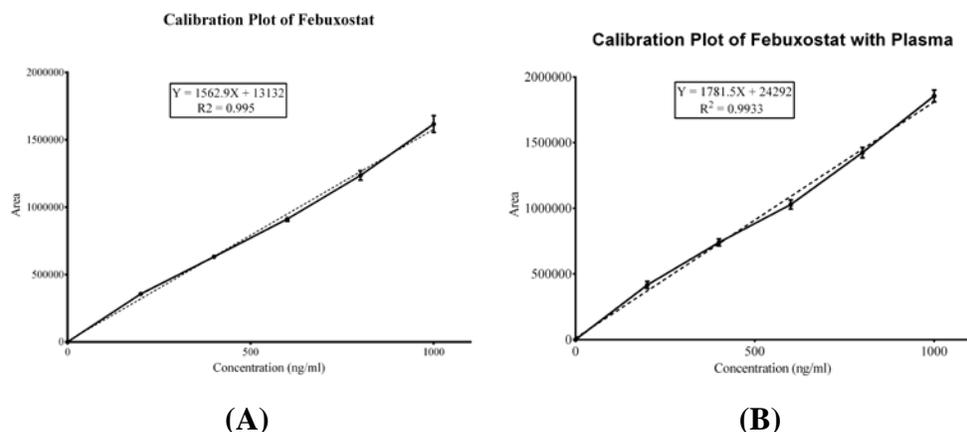
**Figure 3.7: Calibration plot for FBX using HPLC (A) Analytical method
