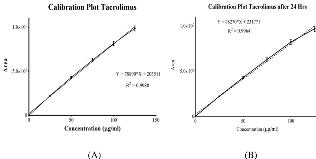
**Figure 3.2: Calibration plot of TAC for analytical method (A) at 0 Hr and (B) after 24 Hr using HPLC analytical method**
