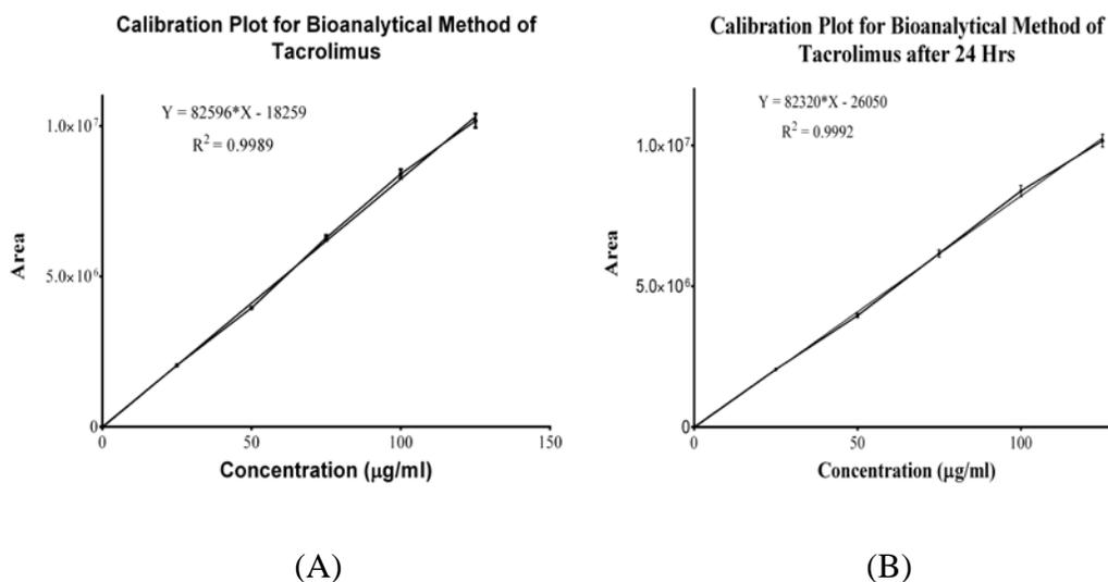
**Figure 3.3: Calibration plot of TAC for bioanalytical method (A) at 0 Hr and (B) after 24 Hr using HPLC analytical method**
