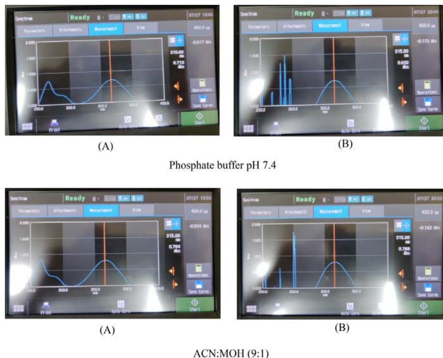
**Figure 3.10: Absorption spectra of FBX (A) without blank cubosomal dispersion (B) in presence of cubosomal dispersion + Lactose to demonstrate specificity of analytical methods**
