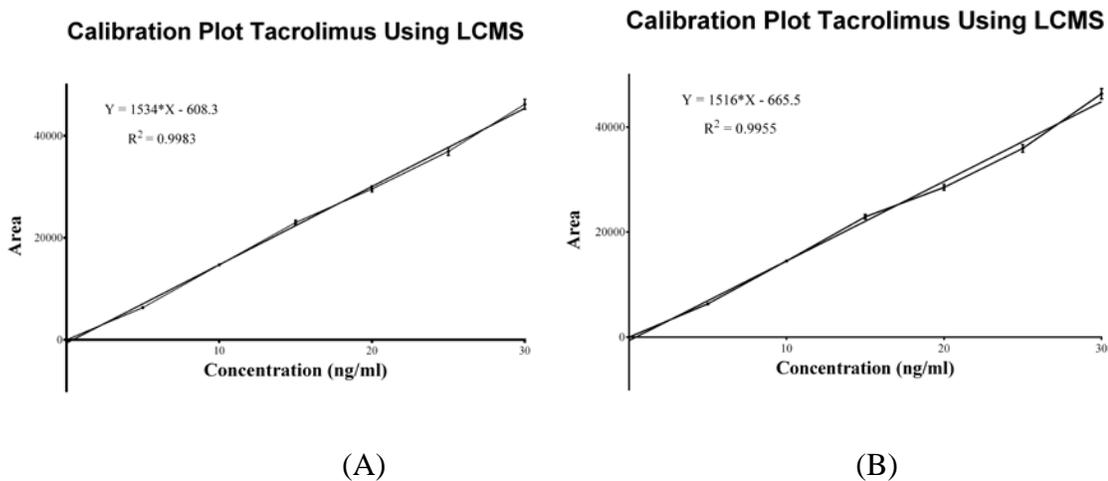
**Figure 3.5: Calibration plot of TAC (A) at 0 Hr and (B) after 24 Hr using LCMS analytical method**
