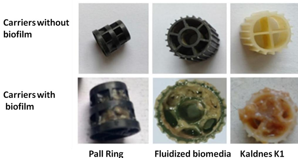
**Figure 3.4 Carriers with different design and surface area used for dMBBR studies**
