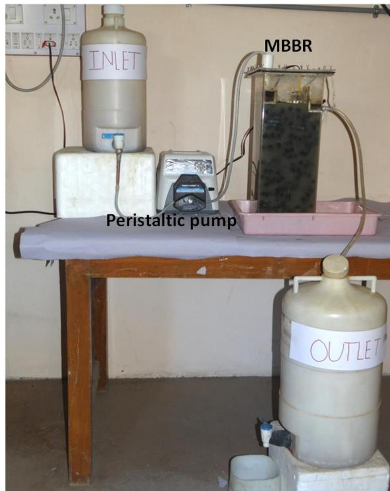
**Figure 3.2 Bench scale dMBBR setup developed with consortium DC5 used in denitrification studies.**
