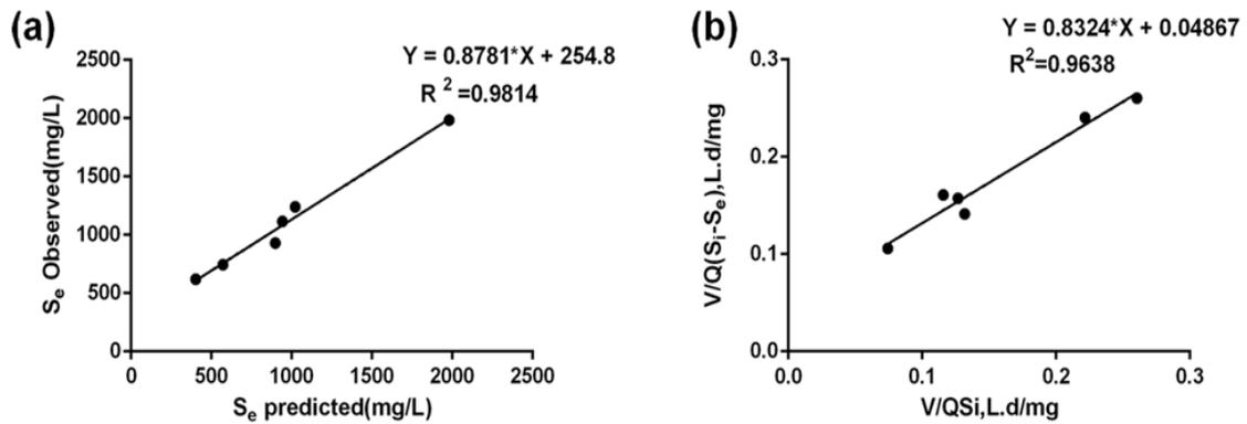
**Figure 3.6 Stover-Kincannon model for denitrifying MBBR (a) Predicted, (b) Observed model**
