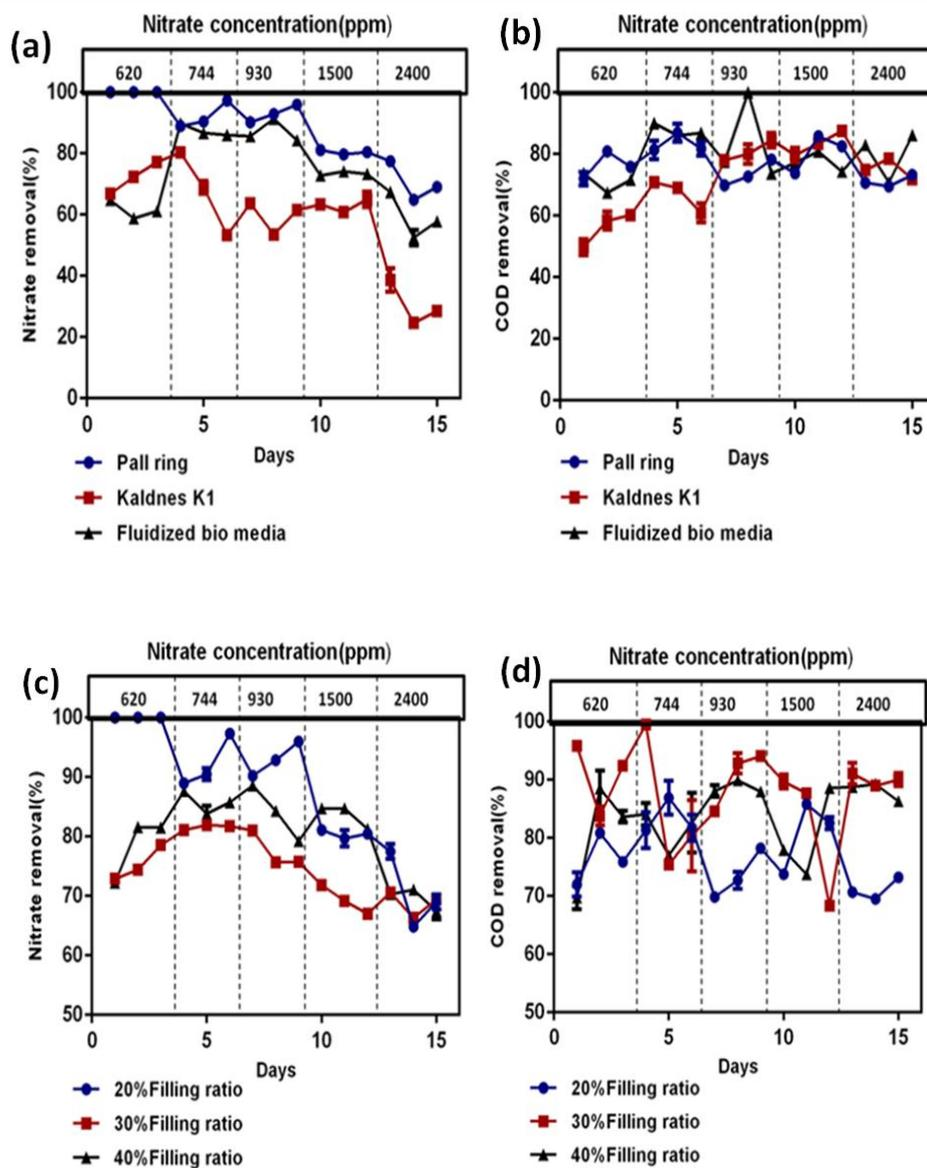
Figure 3.5 dMBBR studies with different carrier design and filling ratio.
