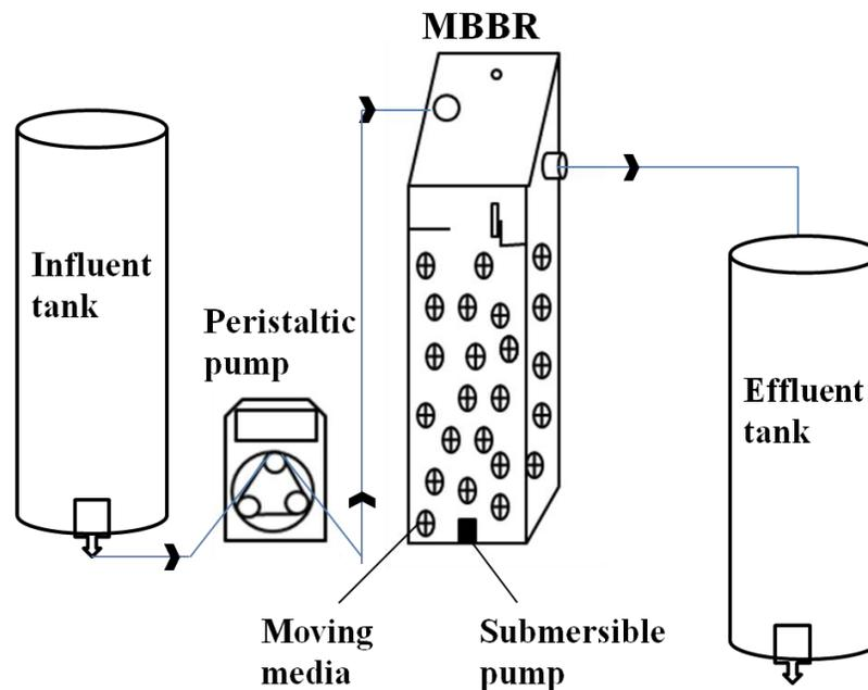
**Figure 3.1** Experimental setup of dMBBR
