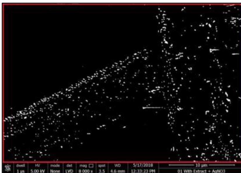
**Figure 4.12: Micrograph used for determination of nanoparticles size distribution [290]**
