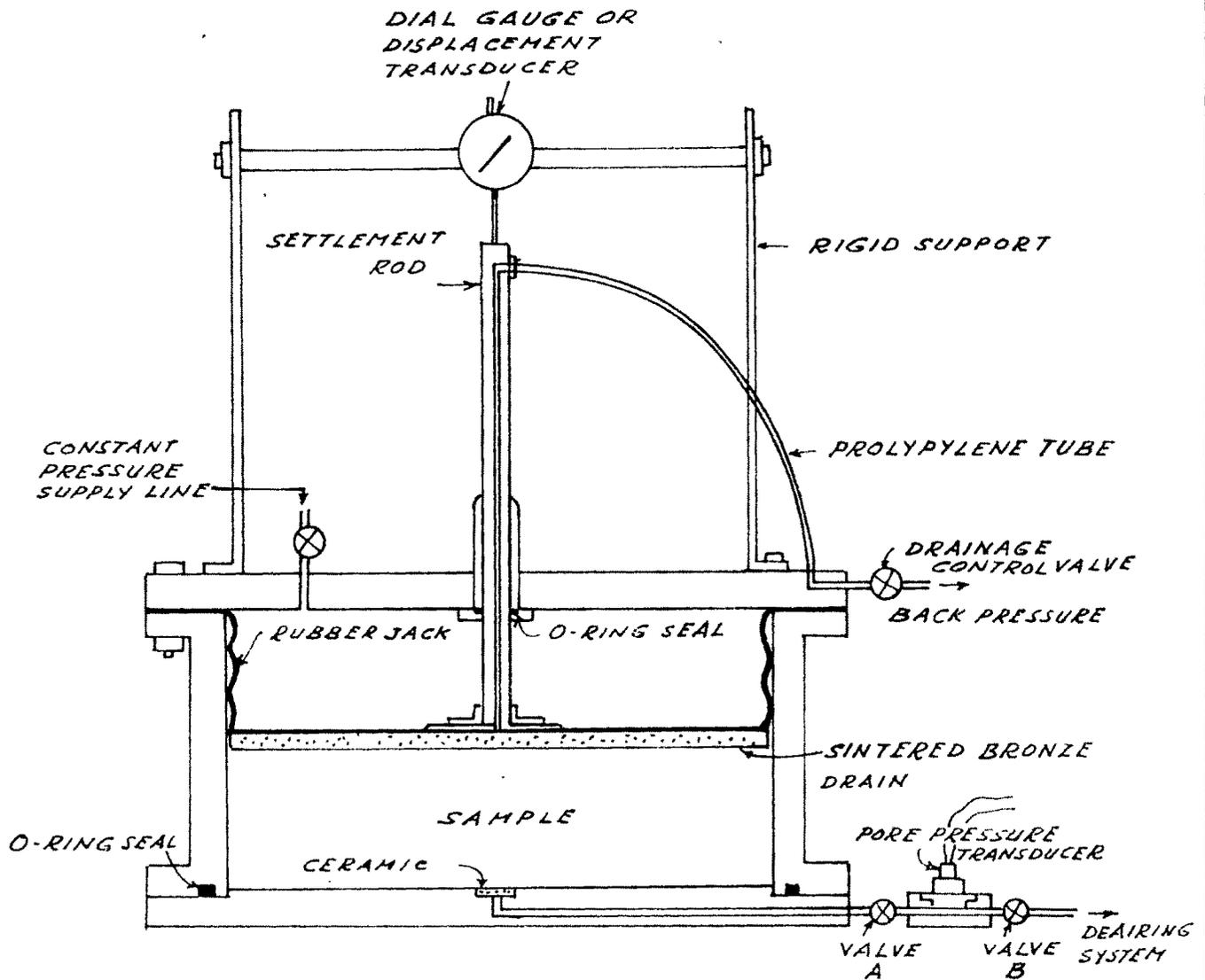
FIG. 6.2 DETAILS OF ROWE OEDOMETER
