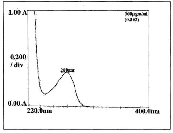
Figure 3.9 Absorptivity scan of leuprolide acetate in PBS (100µg/ml)
