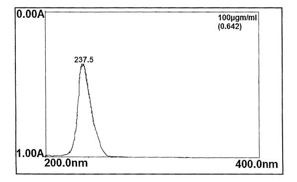
Figure 3.3 Absorptivity scan of cyclosporine in THF/Methanol
