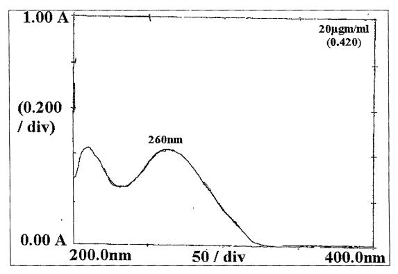
Figure 3.7 Absorptivity of DNA in Tris buffer (20µgm/ml)
