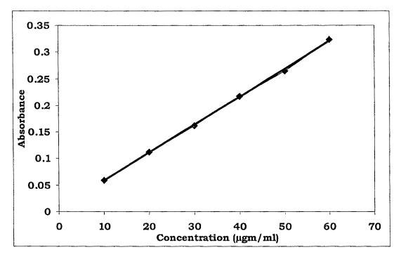
Figure 3.6 Calibration curve for leuprolide acetate in 0.1N NaOH
