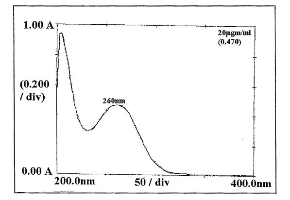
Figure 3.11 Absorptivity scan of DNA in PBS (20µg/ml)
