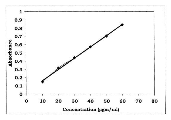
Figure 3.13 Calibration curve for mPEG5000-CC-PE
