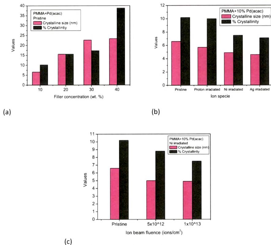
Fig. 6.5 Crystalline size and % crystallinity by XRD analysis as a function of (a) filler concentration (b) ion specie and (c) ion fluence for PMMA+Pd(acac) composites.
