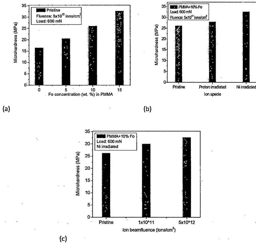
**Fig. 6.4** Vicker's microhardness as a function of (a) filler concentration and (b) ion specie and (c) ion fluence at a load of 600 mN
