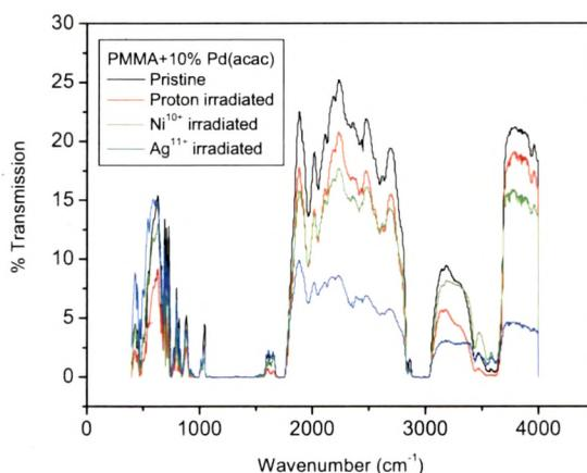
**Fig. 6.6 FTIR spectra for pristine and irradiated films of PMMA+10%Pd(acac)**
