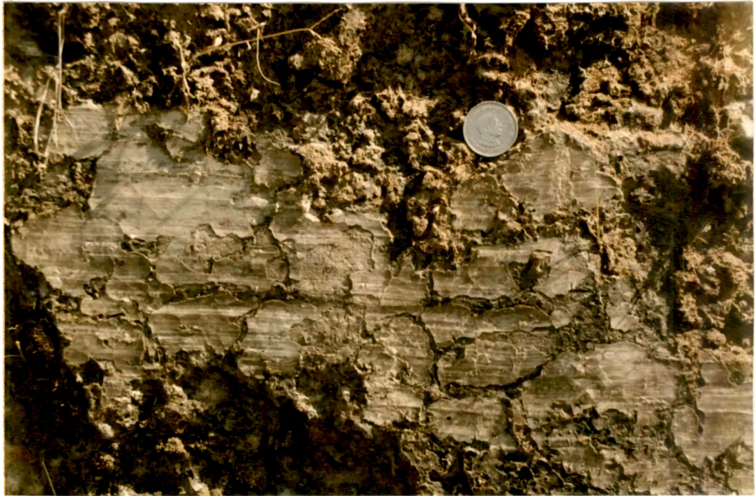
Plate 4.1 : Close-up view of slickensides on the exposed face of the silty-sand unit at Kadana.
