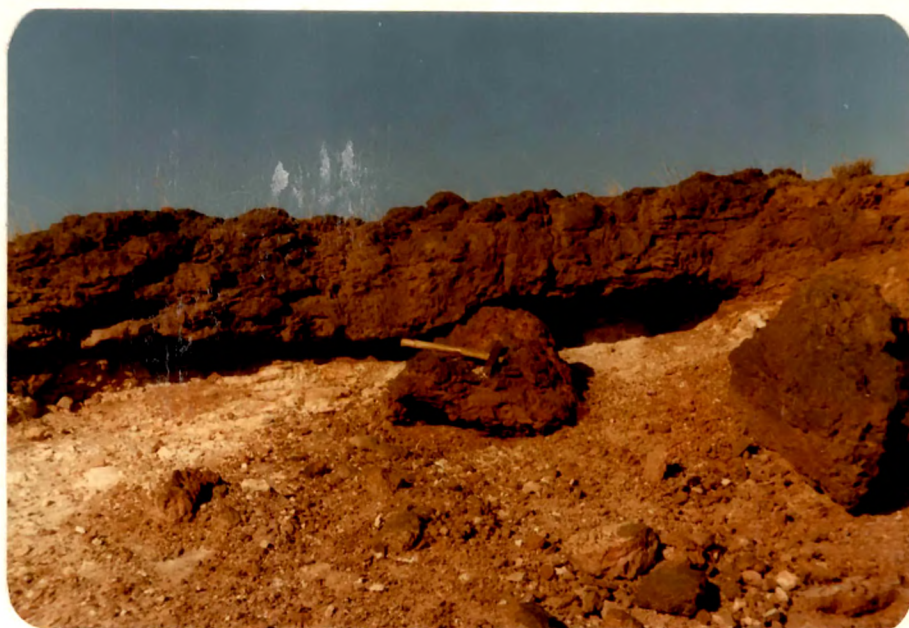
Plate 3 : Typical LST type of section depicting laterite/ bauxite underlain by only kaolinite.
