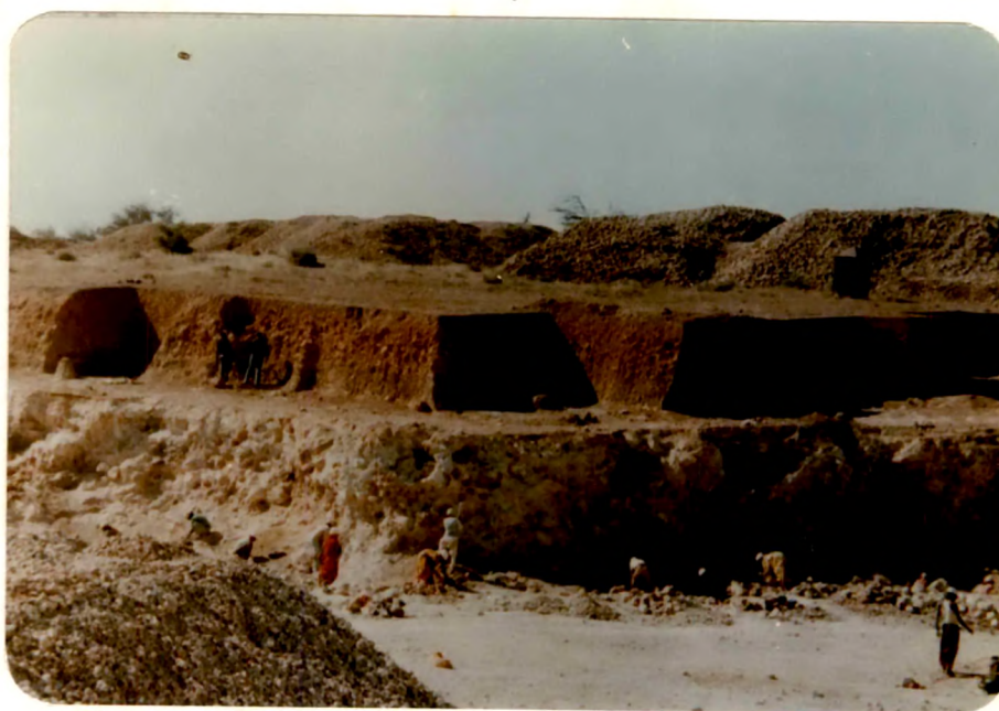
Plate 2 : Typical HST type of section showing laterite/ bauxite, kaolinite, bentonite and Deccan Trap basalt in one gradational section.
