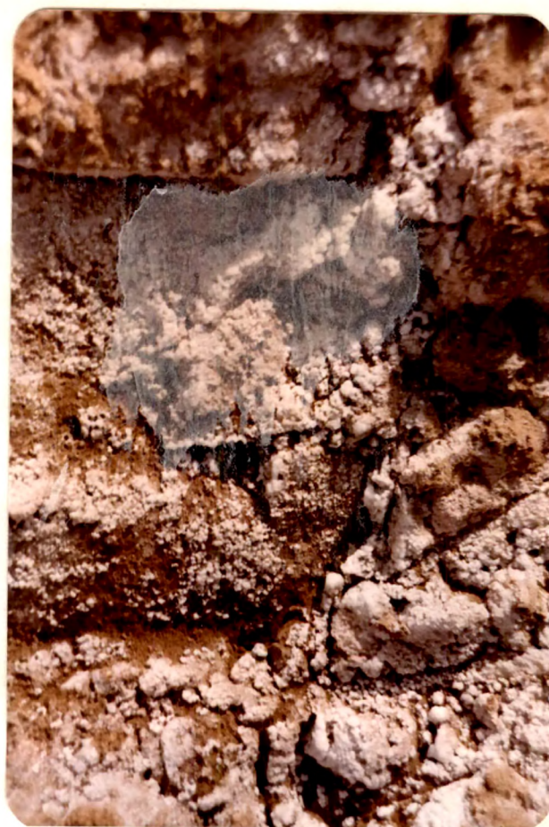
Plate 10 : The bentonite layer is nearly always traversed by numerous thin veins and encrustations of calcite and gypsum.
