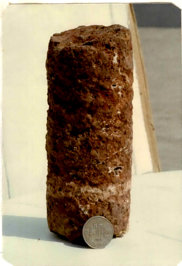
Plate IV.23 Core of duricrust showing numerous cavities with layers of Al and calcareous materials from Pavdi bore hole.
