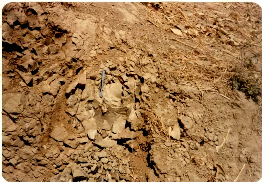
Plate IV.50 Typical spheroidal weathering in basalt at the base of laterite profile near Khutai Mata temple.
