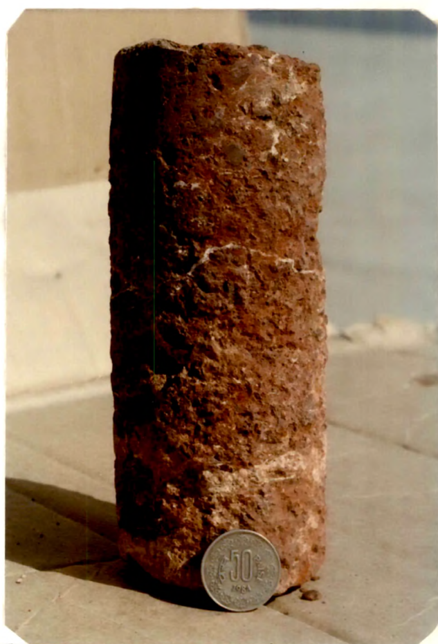
Plate IV.23 Core of duricrust showing numerous cavities with layers of Al and calcareous materials from Pavdi bore hole.
