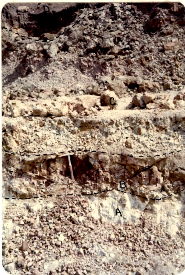
Plate IV.45 Exposed section in quarry at Vagalkhod. A. Kaolinite B. Lithomarge C. Reworked laterite & bauxite D. Black cotton soil.
