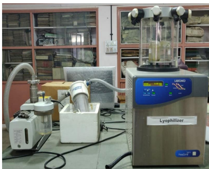
Figure 3.4: Lyophilizer used for the lyophilisation of the aqueous extract
