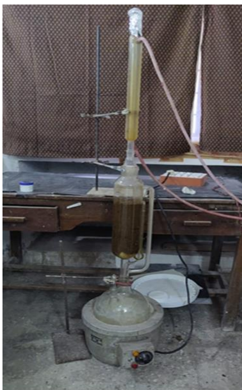
Figure 3.3: Soxhlet extraction setup used for extraction of phytochemicals from B. variegata leaves.
