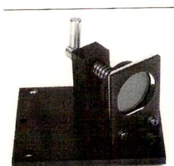
Fig.3.4 Spectrofluorophotometer Powder Sample Holder
