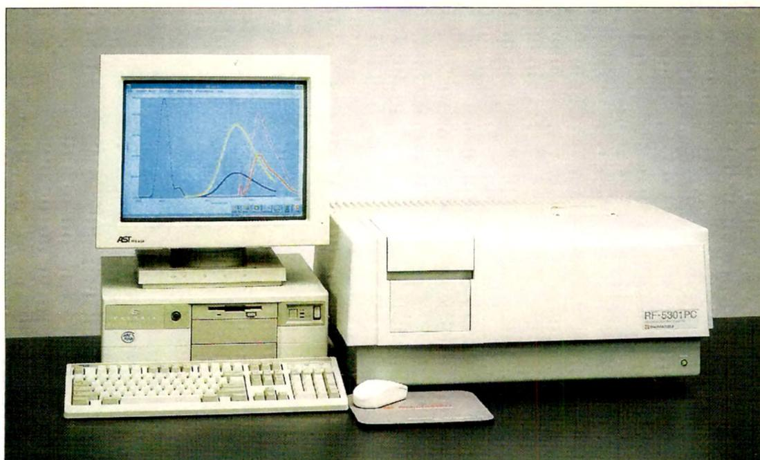
Fig. 3.3 Spectrofluorophotometer, RF-5301PC
