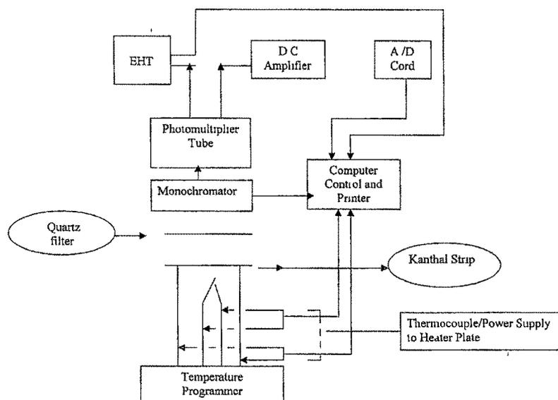
**Fig.3.8 TL Emission Equipment Set-up**
