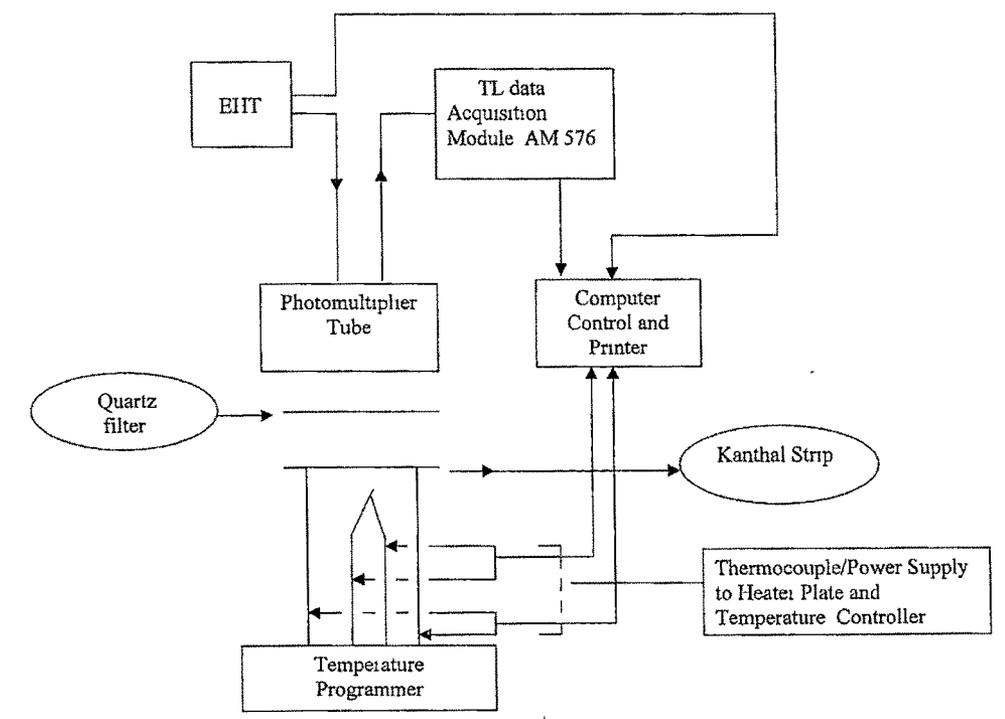
**Fig.3.7 Block Diagram of TL Set-up**
