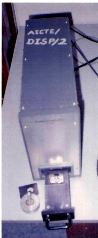
Fig.3.5 Thermoluminescence Setup
