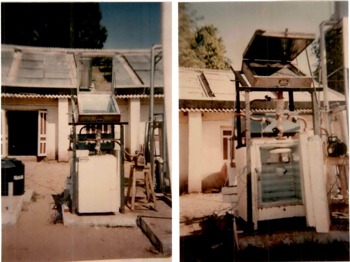
Fig. 7.2 : Solar refrigerator (left) during day cycle,
