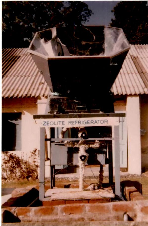
Fig. 7.6 : Prototype with eight sided booster arrangement
