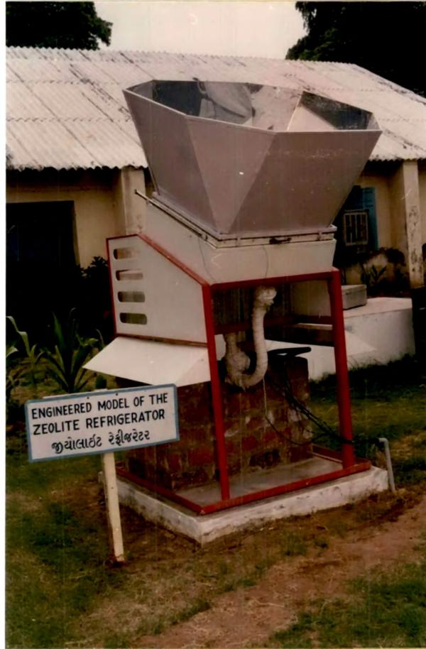
Fig. 7.7 : Engineered prototype of the solar refrigerator
