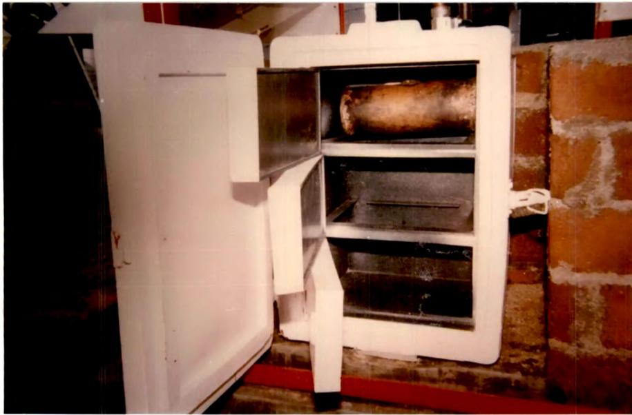
Fig. 7.10 : Cold box and the evaporator
