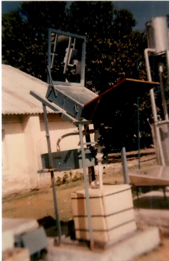
Fig. 7.4 : Two mirror booster arrangement for solar refrigerator
