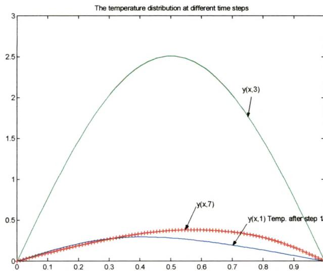
Figure 6.5: The evolution of the temperature distribution at different time-step due to the ANN zonal controller.
