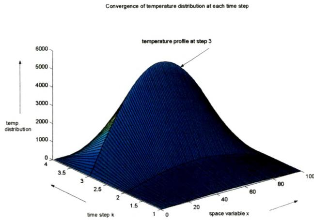
Figure 6.7: The evolution of the temperature profile due to the 4-step ANN zonal controller.
