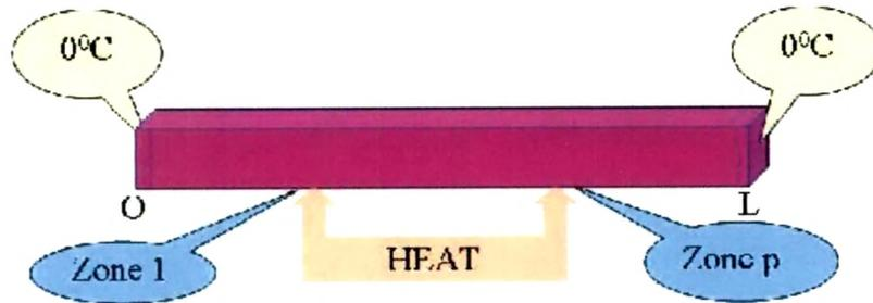
Figure 6.1: Conductive bar coated with more conductive material on the lateral sides
