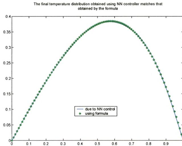
Figure 6.4: The final temperature distribution steered due to the control signal produced by ANN Zonal Controller and the desired temperature distribution.
