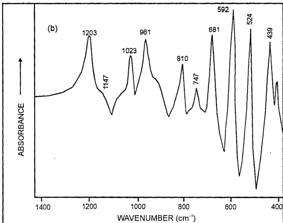
Figure 5.12: FT-IR spectra of green beryl. a) normal FT-IR spectra b) FSD trace of green beryl
