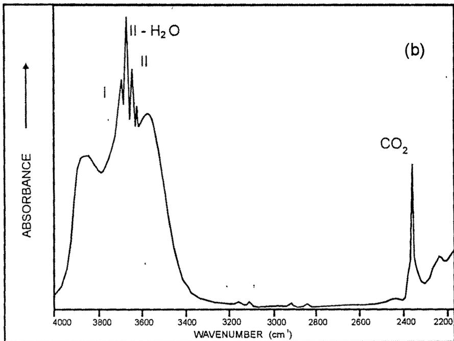
Figure 5.6 : Single crystal FT-IR spectra of (a) Tamil Nadu (Karur) and (b) Kerala green beryl indicating more of type-II water molecules in green beryl compared to blue beryl.
