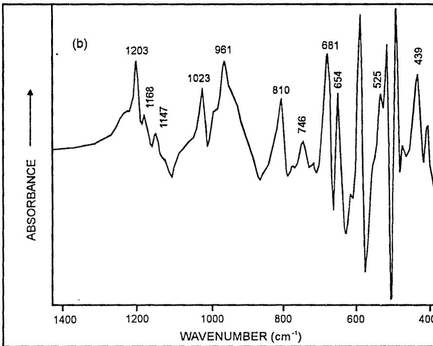
Figure 5.11 : FT-IR spectra of blue beryls. a) normal FT-IR spectra and b) FSD trace of blue beryl.
