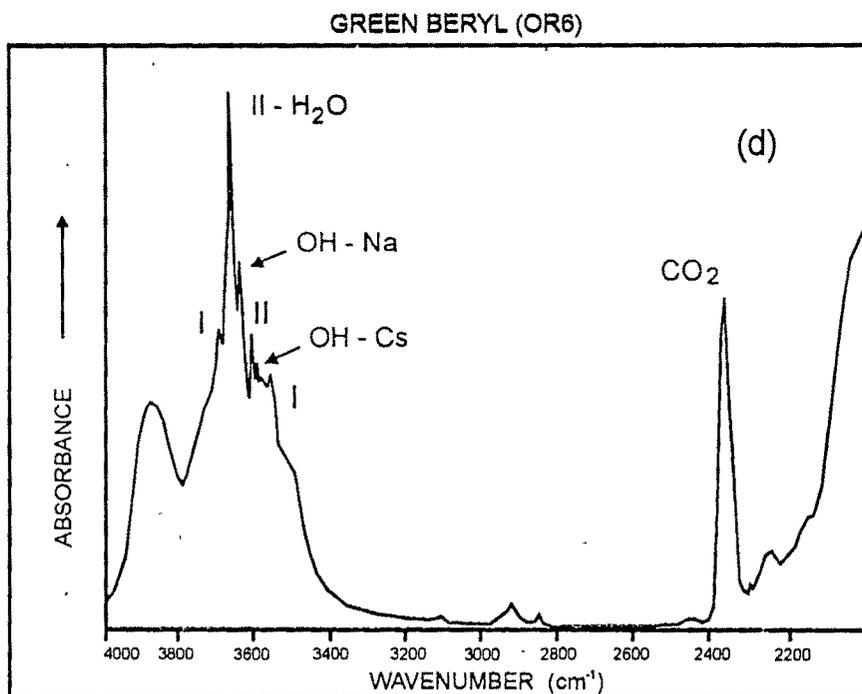
Figure 5.5 : Single crystal FT-IR spectra of (c) blue and (d) green beryl depicting presence of various hydrous species and CO<sub>2</sub> molecules in the channel site. Green beryl shows predominance of type-II H<sub>2</sub>O molecule compared to other coloured beryls
