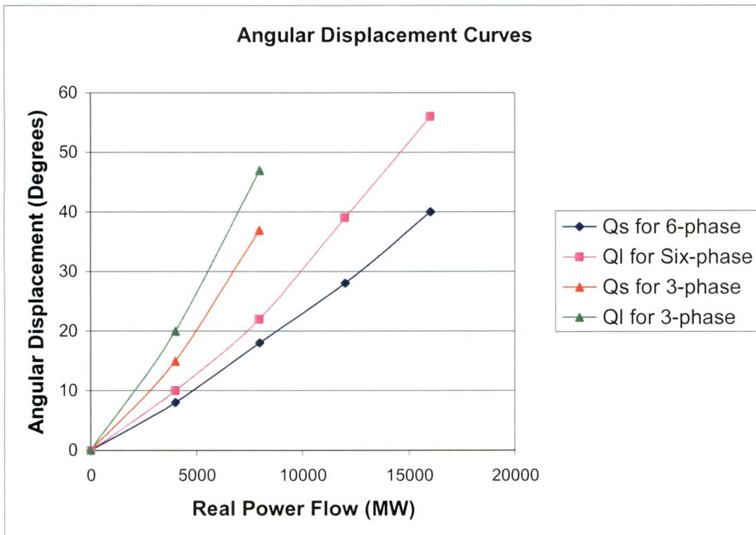
Fig. 4.14 Angular Displacement Curves GETCO’s 400KV three-phase Double Circuit Line and Its Conversion to Six-phase
