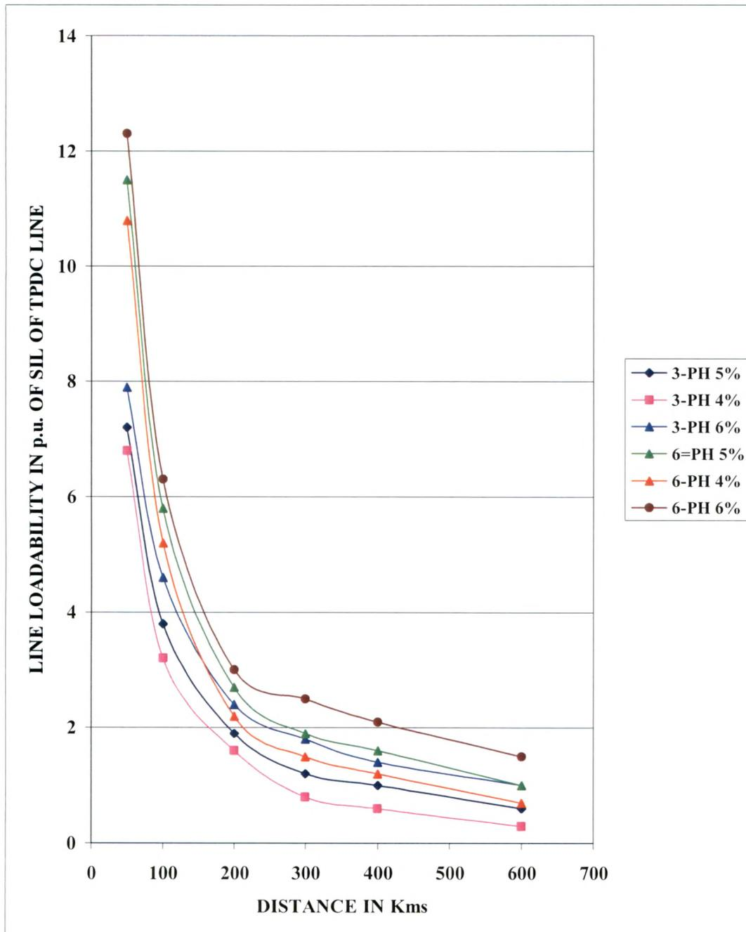
Fig. 4.9 Effect of Voltage drop Limit on Line Loadability
