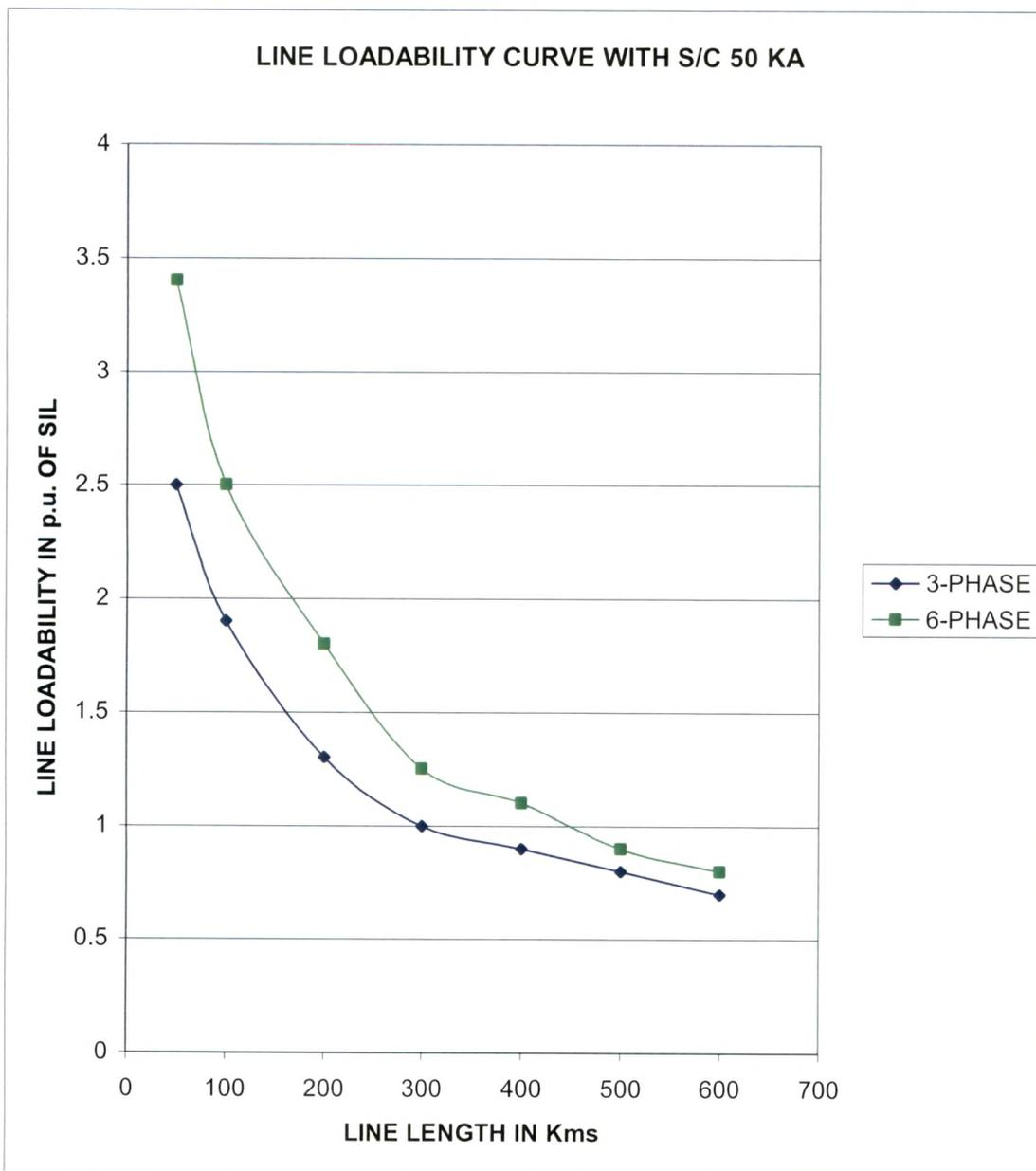
Fig. 4.5 Loadability curves for 400 KV alternative lines.
