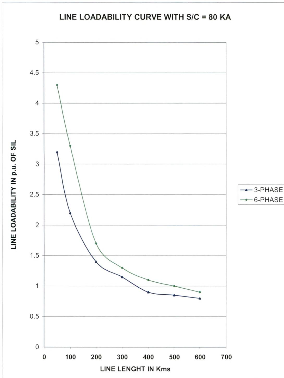
**Fig. 4.4** Generalized loadability curves for 400 KV alternative lines.
