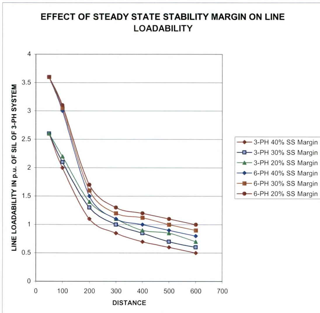
**Fig. 4.10 Effect of Variation of Steady State Stability Margin, on Line Loadability for 3-phase and 6-phase Transmission Systems.**
