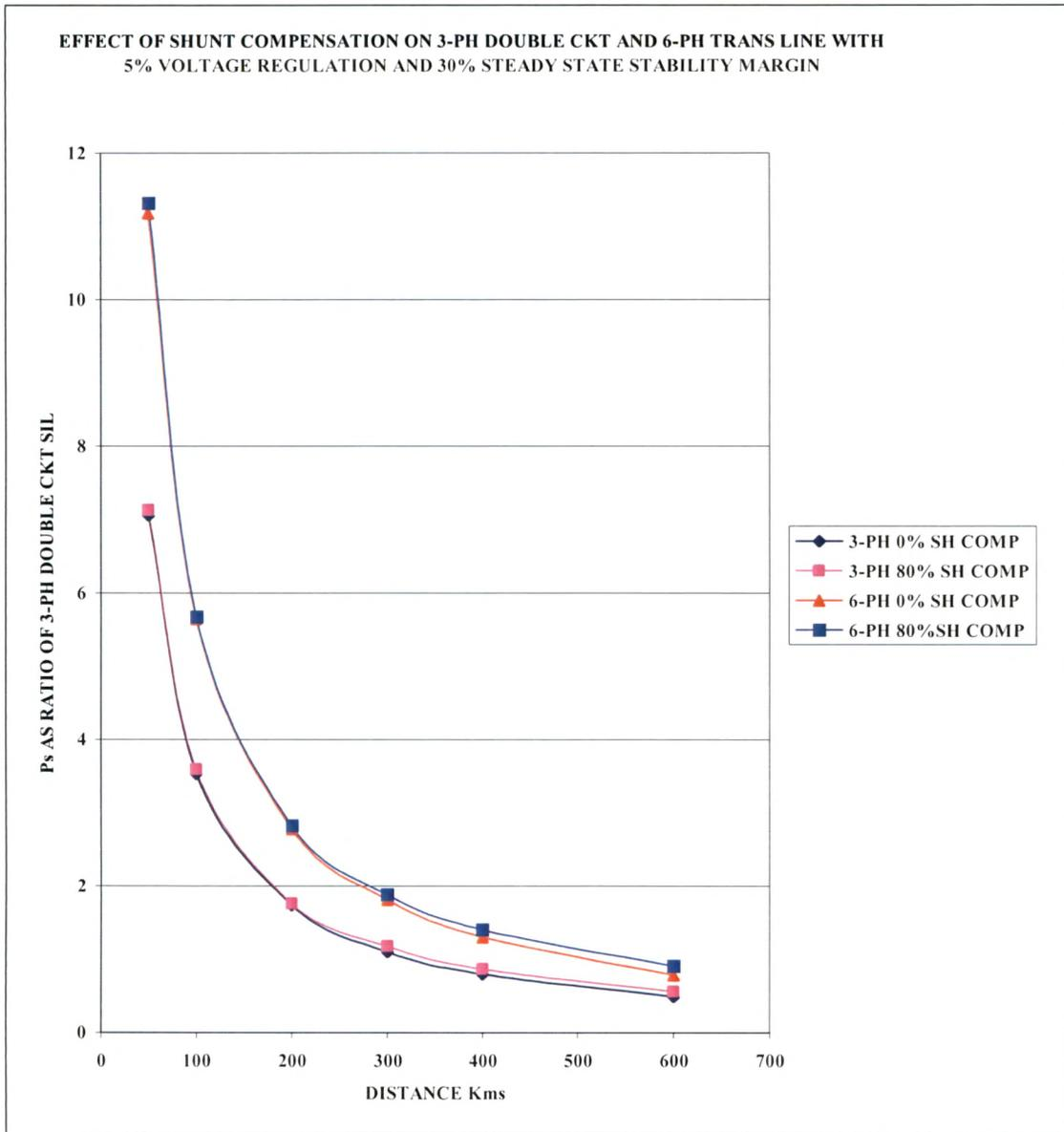
**Fig. 4.6 Effect of Shunt Compensation on Line Loadability**
