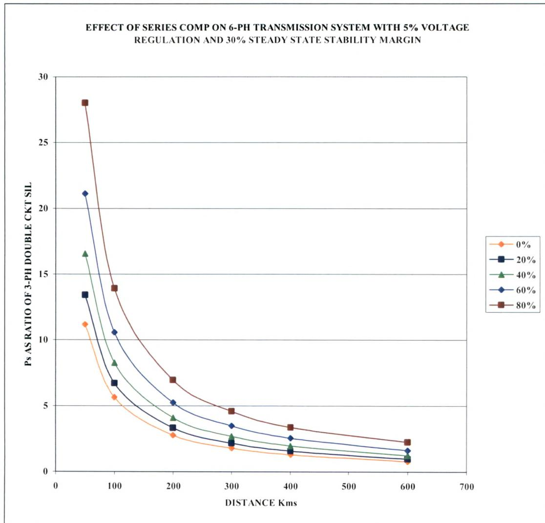
**Fig. 4.8 Effect of Series Compensation on (GETCO'S three-phase Double Circuit Line Converted in to Six-phase) Six-phase Line Loadability**
