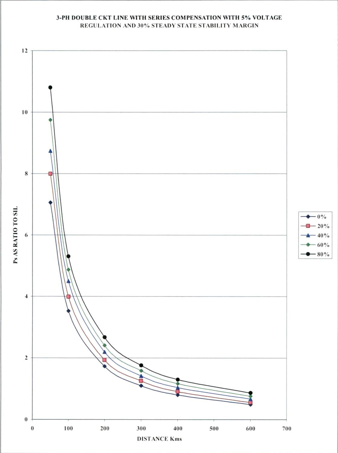
**Fig. 4.7 Effect of Series Compensation on GETCO'S three-phase Double Circuit Line Loadability**
