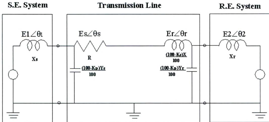
(  $K_s / K_p$  : Degree of series and shunt compensation)
