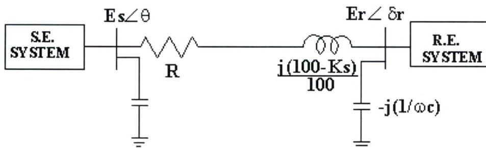
Fig:4.3 A Line Model for Loadability Dependence on Var Supply
