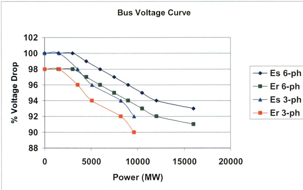
Fig. 4.13 Bus Voltage Curves for GETCO’s 400KV three-phase Double Circuit Line and Its Conversion to Six-phase
