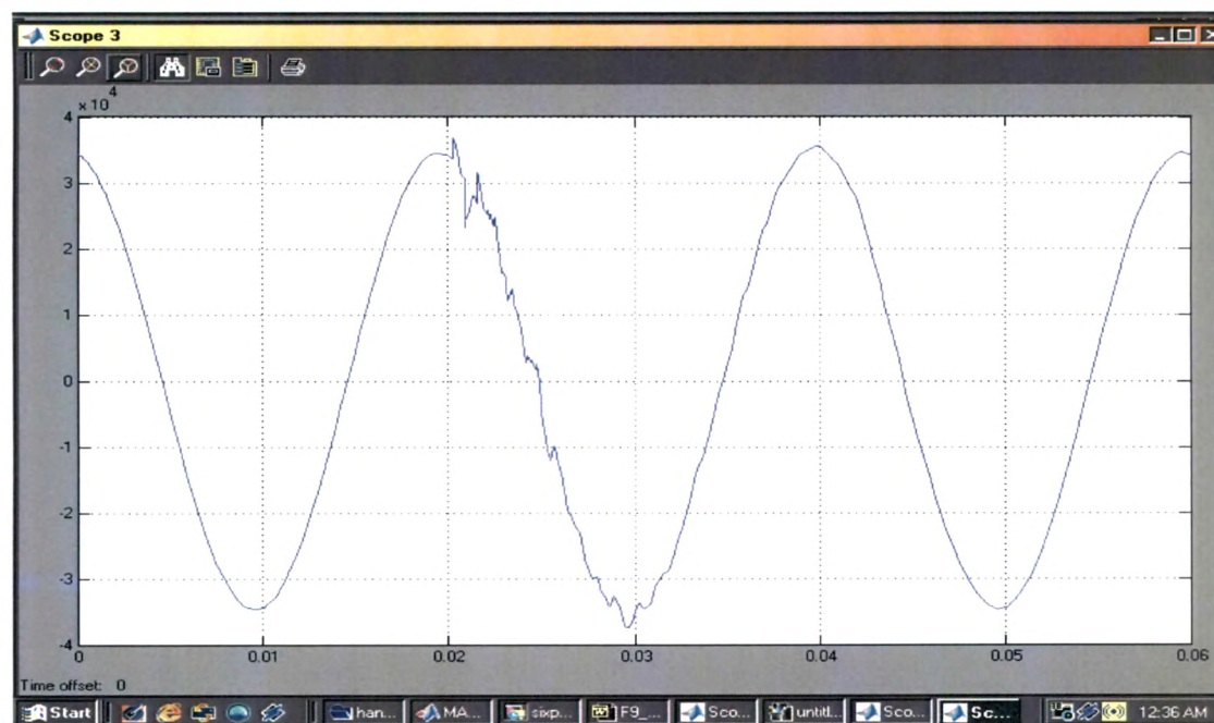
Load Side Phase Voltage on Single Line to Ground Fault at mid-point on 6-phase
