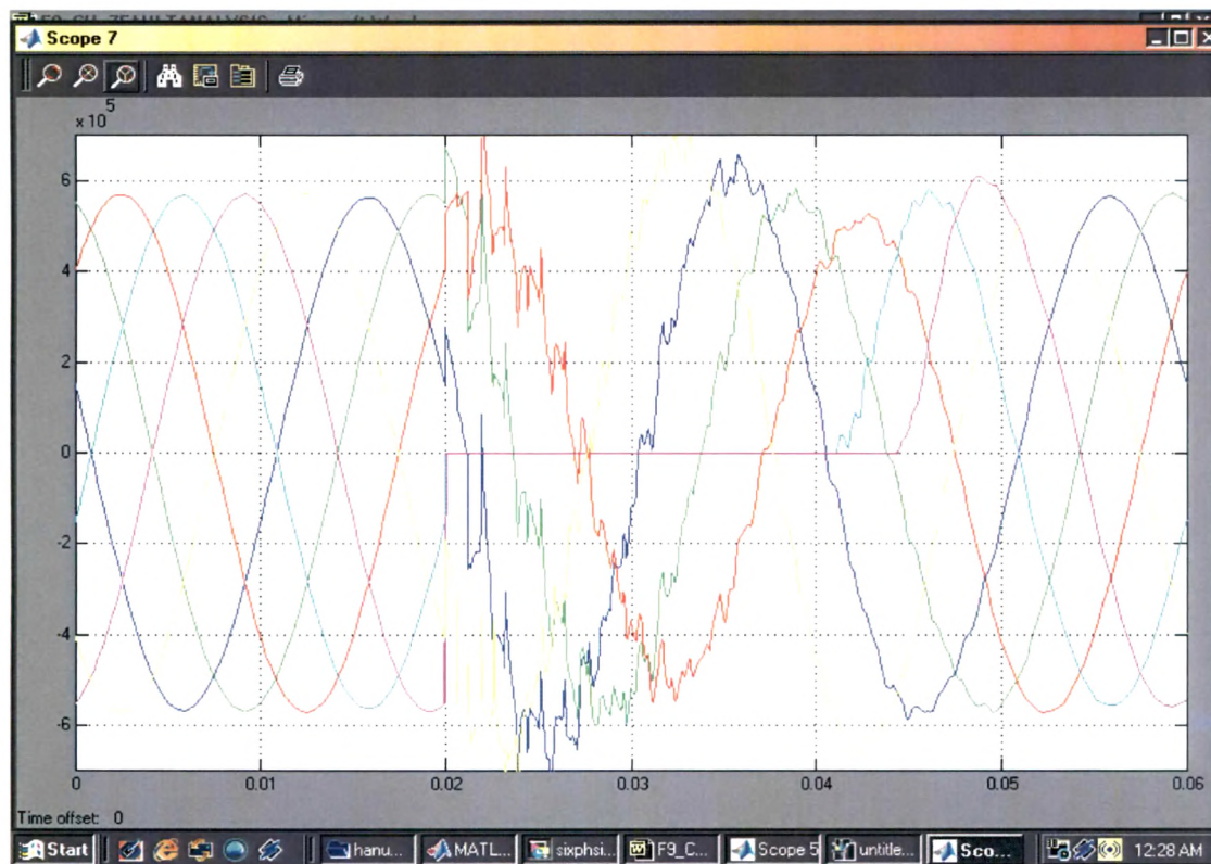
Fault Voltages for fault Double Phase to Ground in Six-Phase at Mid-point
