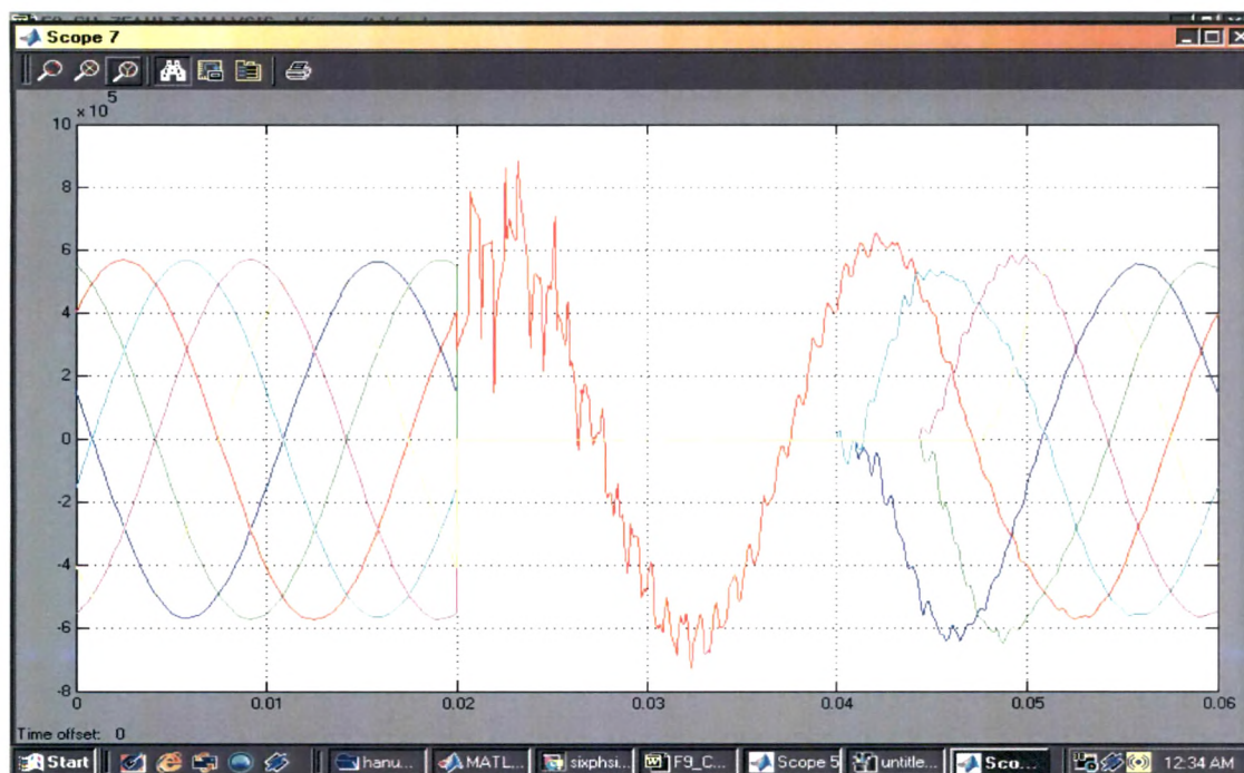
Fault Voltages for fault Five Phase to Ground in Six-Phase at Mid-point
