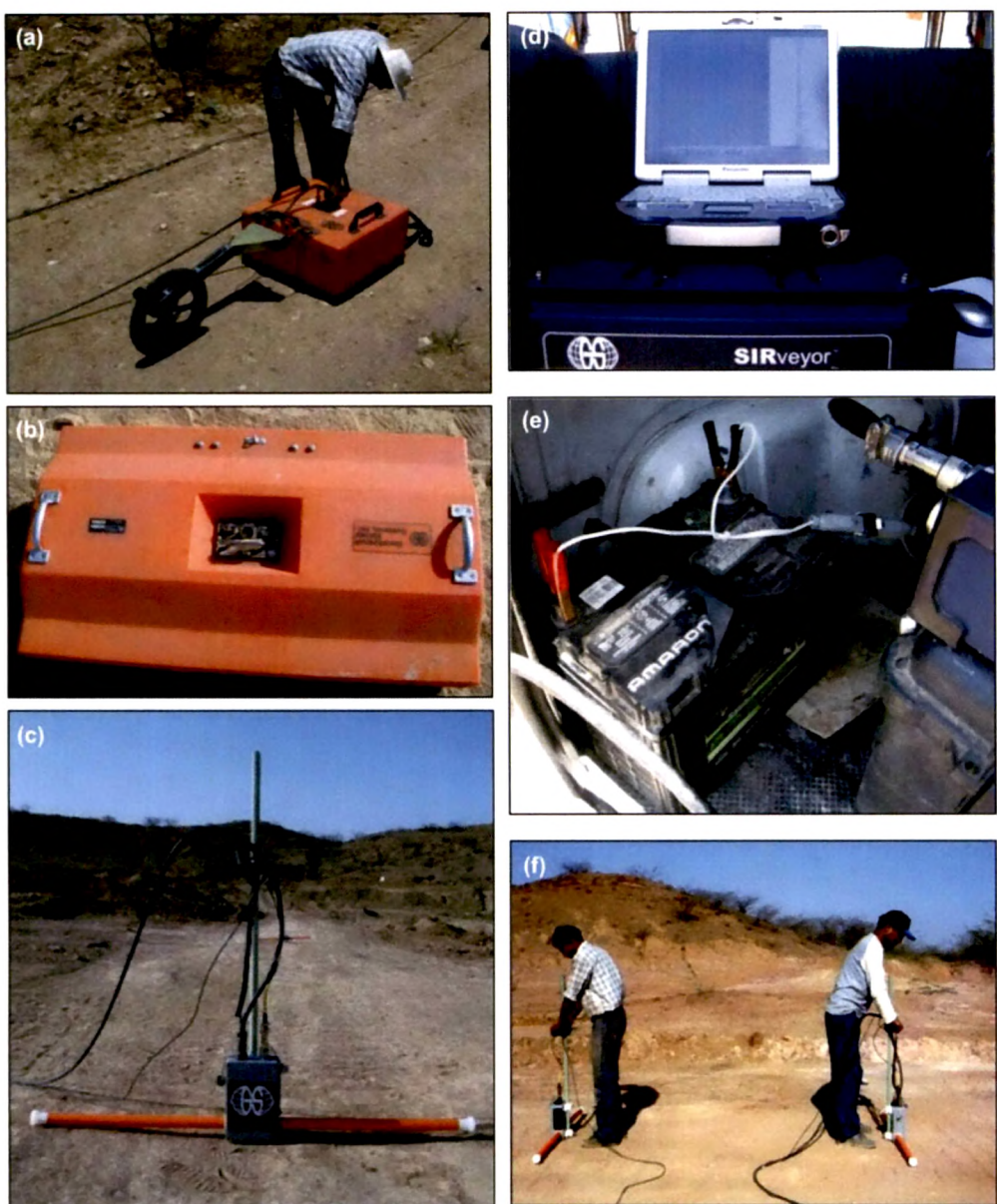
Figure 5.3 The SIR-20 GPR system used in the present study with all necessary accessories manufactured by the Geophysical Survey Systems Inc. (GSSI), USA. (a) 200 Mhz shielded antenna (b) 100 Mhz shielded paired antenna (c) Multi-Low Frequency (MLF) antenna (80-15 Mhz) (d) GPR Main operating unit (e) 12V Battery (power source) (f) Transmitter and receiver units of MLF antenna with transmission cable.
