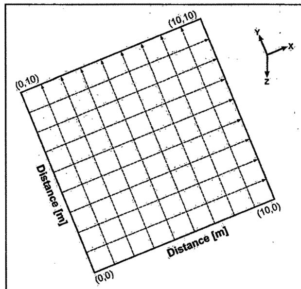
**Figure A.1** The survey planning for 3D GPR data acquisition.
