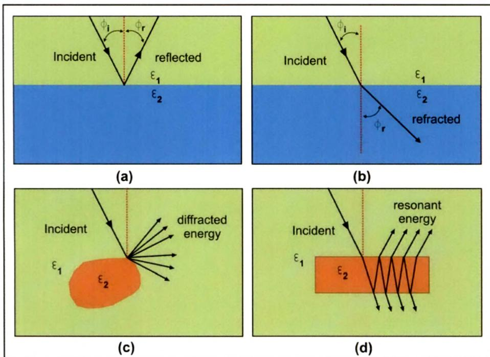
**Figure A.2** General scattering patterns for radar and seismic waves. (a) Specular scattering (b) Refraction scattering (c) Diffraction scattering (d) Resonant scattering (after Daniels, 2000).
