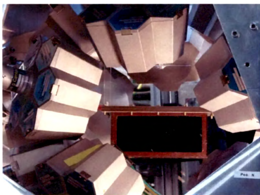
Figure 7.15: The Cluster array of the stopped beam RISING experiments with the active stopper vessel made out of Pertinax (left) and the top cover of the active stopper chamber with the cable connectors (right) for six DSSSD arranged in two rows.
