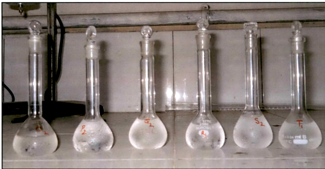
Plate 4.3.4.1.4.3.1: Dilution of oil sample with isooctane in 25 ml volumetric flask
