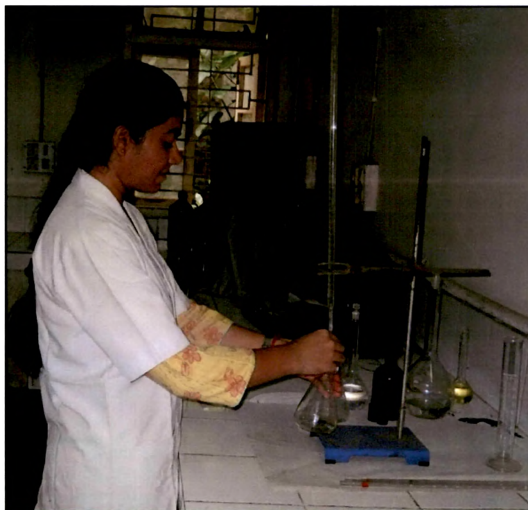
Plate 4.3.4.1.3.3: Determination of peroxide value by titration method
