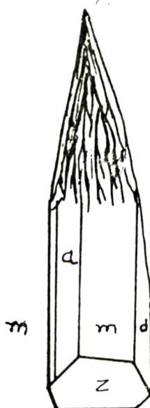
Fig. 4.5 (b) Schematic diagram of a needle shaped crystal.
