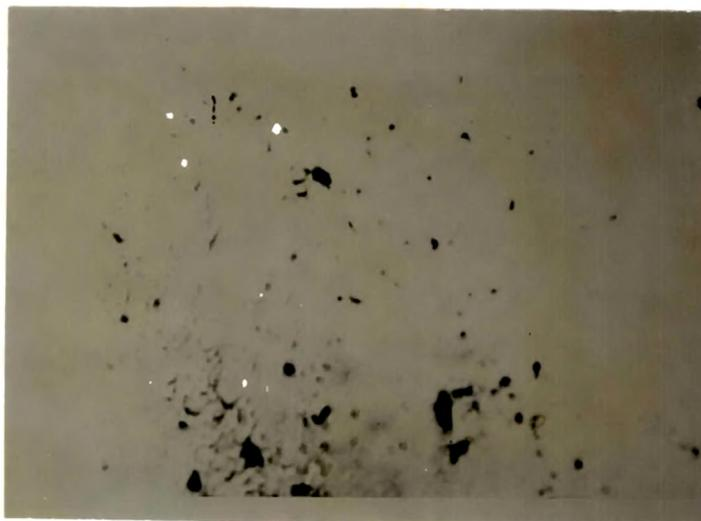
Fig.4.11 (a) - Photomicrograph of as-grown z-face (111) with ammonium bromide as the feed solution.
