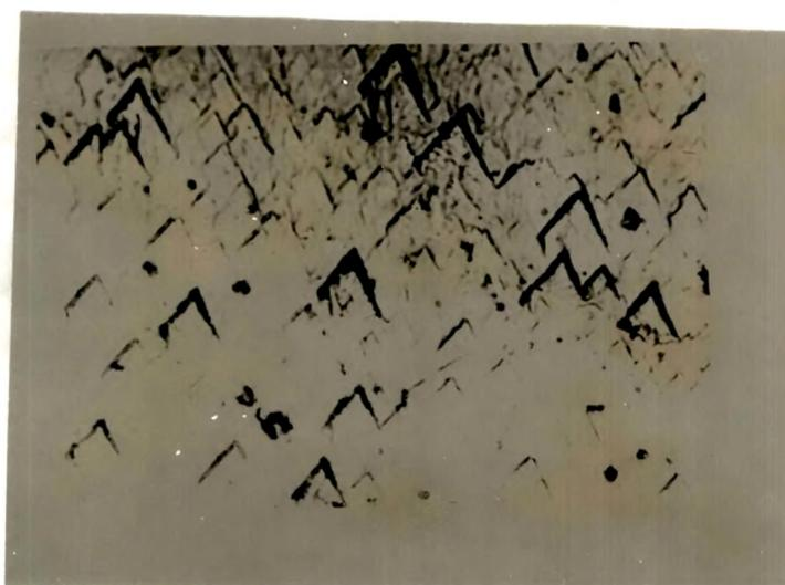
Fig.4.11 (b) - Photomicrograph showing the inherent etching of the growing crystal on the as-grown z-face (111) using ammonium chloride as feed solution.
