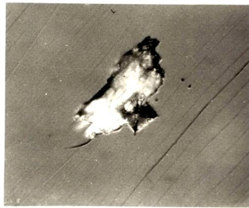
Fig. 7.7 Vickers indentation mark along  $[100]$  on calcite cleavage (P = 80 gm.)
