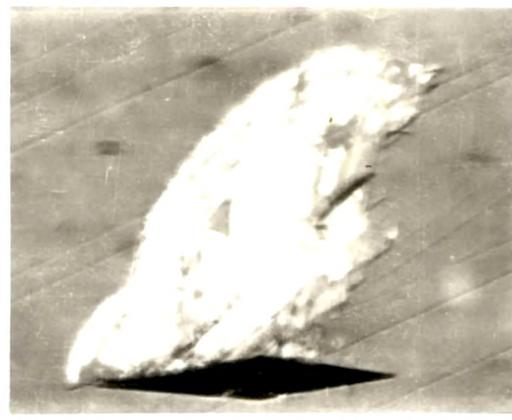
Fig. 7.6 Knoop indentation mark along ~~on~~  $[100]$  on calcite cleavage face. (P = 80 gm.)
