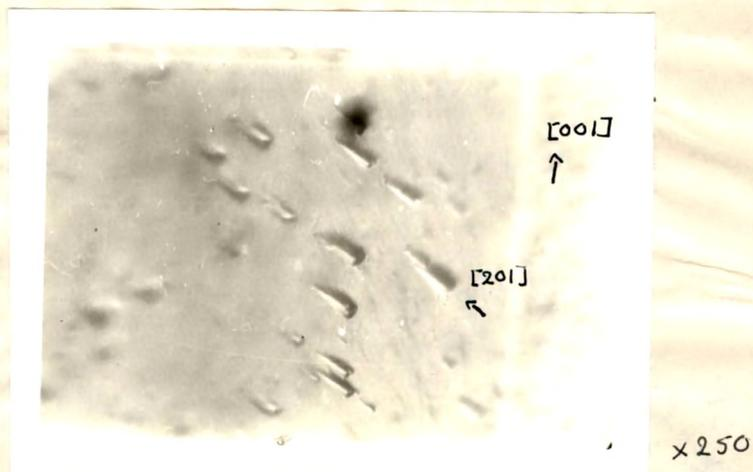
Fig. 8.10 Triangular etch pits on cleavage plane, obtained by etchant 10 gm trichloroacetic acid in 100 c.c. glacial acetic acid for 90 sec. at 30°C.
