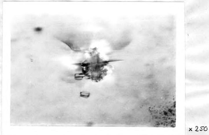
Fig. 10.15 (a) Photomicrograph of d-AlH cleavage surface indented by using vickers hardness indenter by for applied load of 40 g, showing the formations of wings, crystallographic cracks and slip lines.
