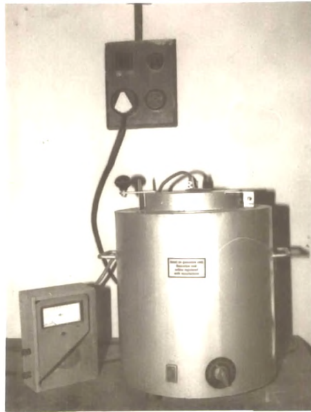
Fig. 2.9 Vertical temperature gradient crucible furnace
