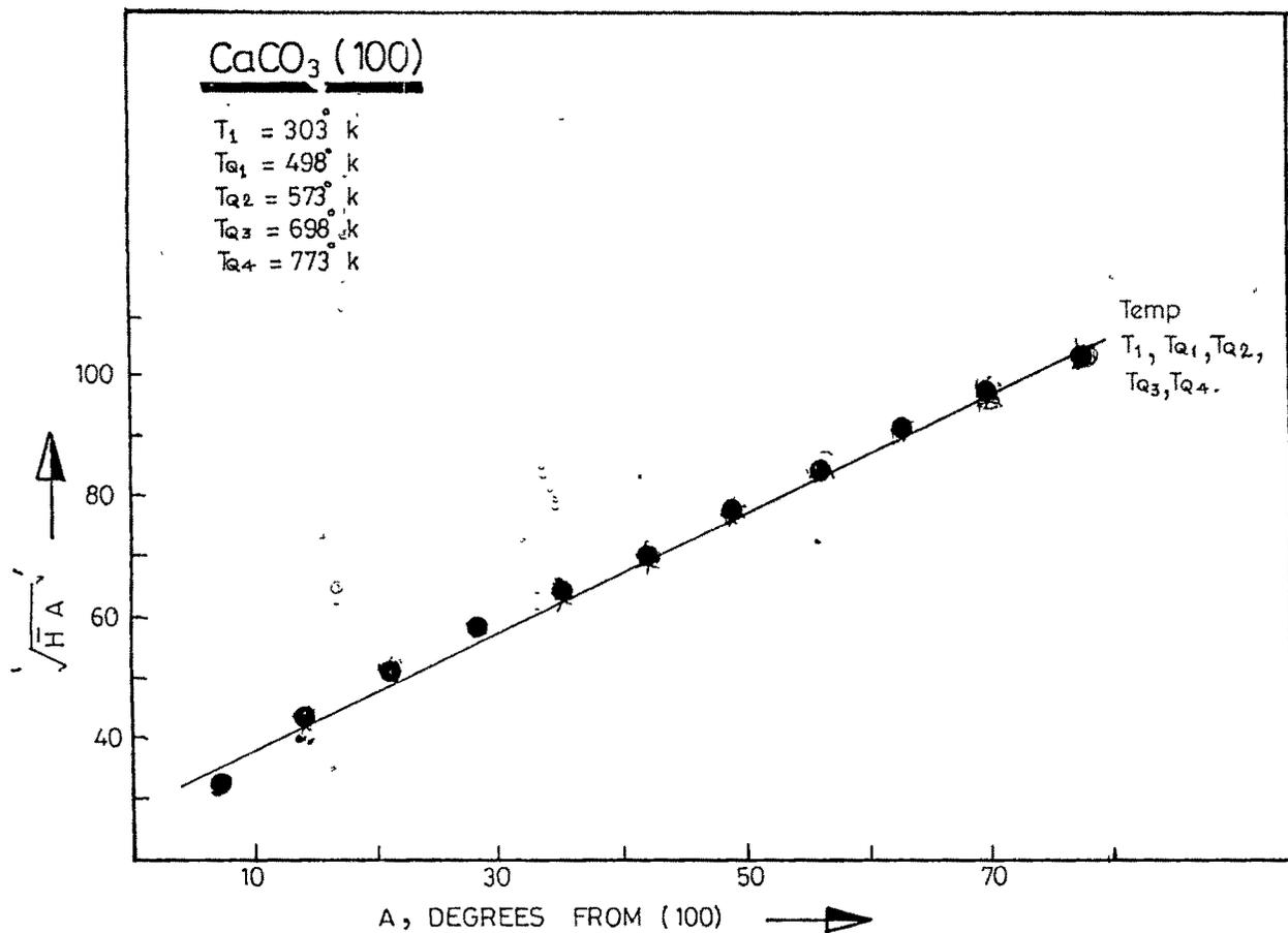
Plot of  $\sqrt{HA}$  vs A, for (100) at room temp.  $T_1$
