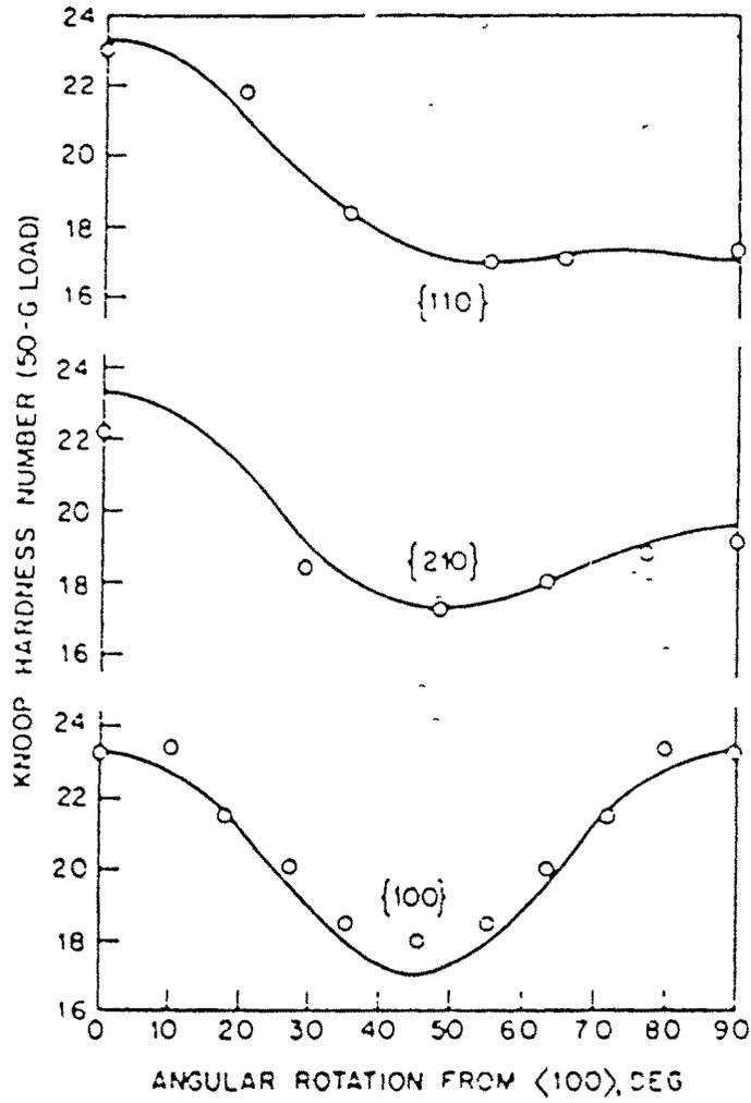
Theoretical and experimental Knoop hardness anisotropy for three crystallographic planes in aluminum as a function of long-axis orientation.
