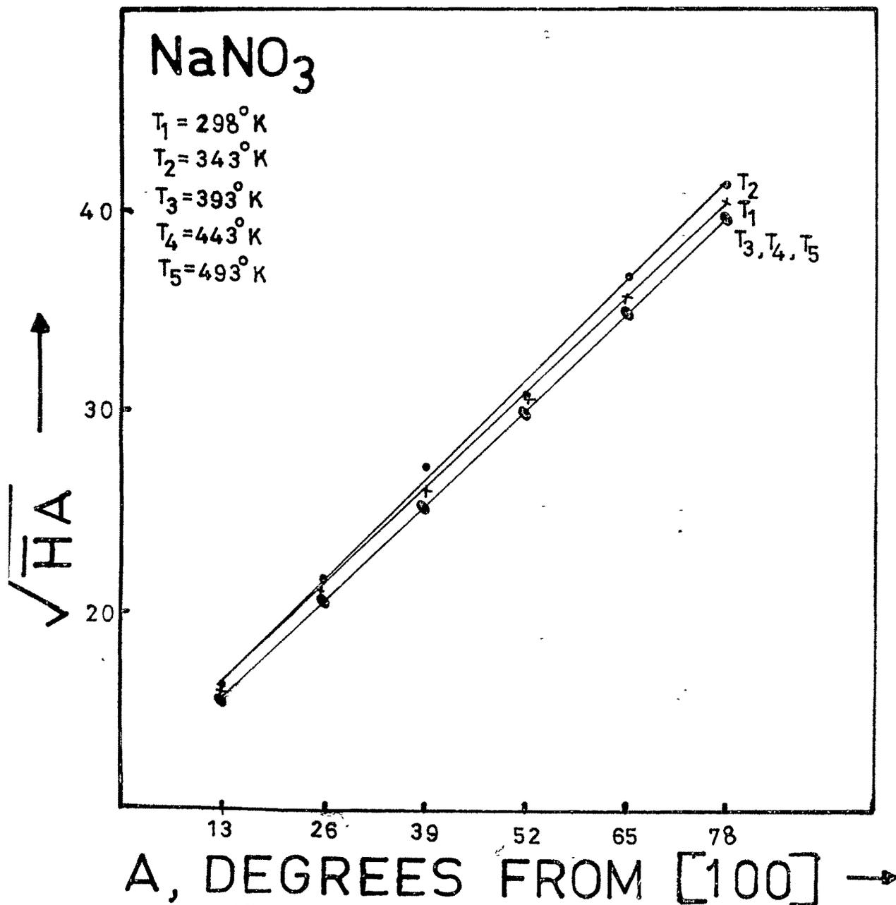
PLOT OF  $\sqrt{HA}$  VS A FOR (100) AT ROOM TEMPERATURE  $T_1$  AND QUENCHING TEMPERATURES  $T_2, T_3, T_4, T_5$ .
