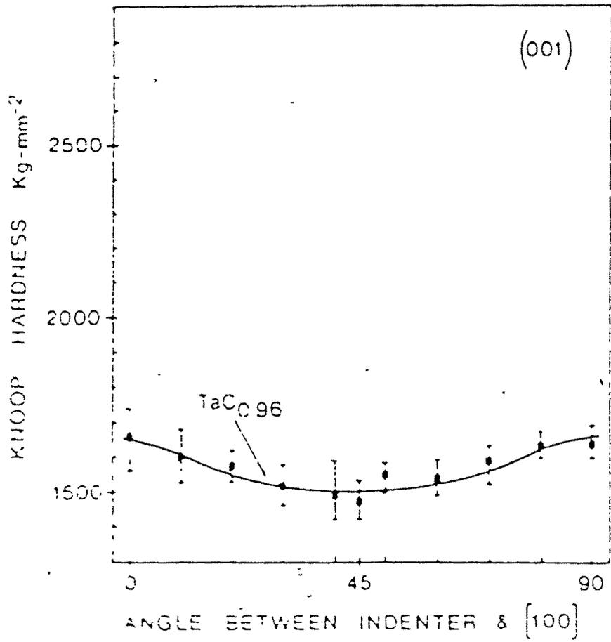
Variation of Knoop hardness (100-gram load) with indenter orientation on (100) surface of TaC.
