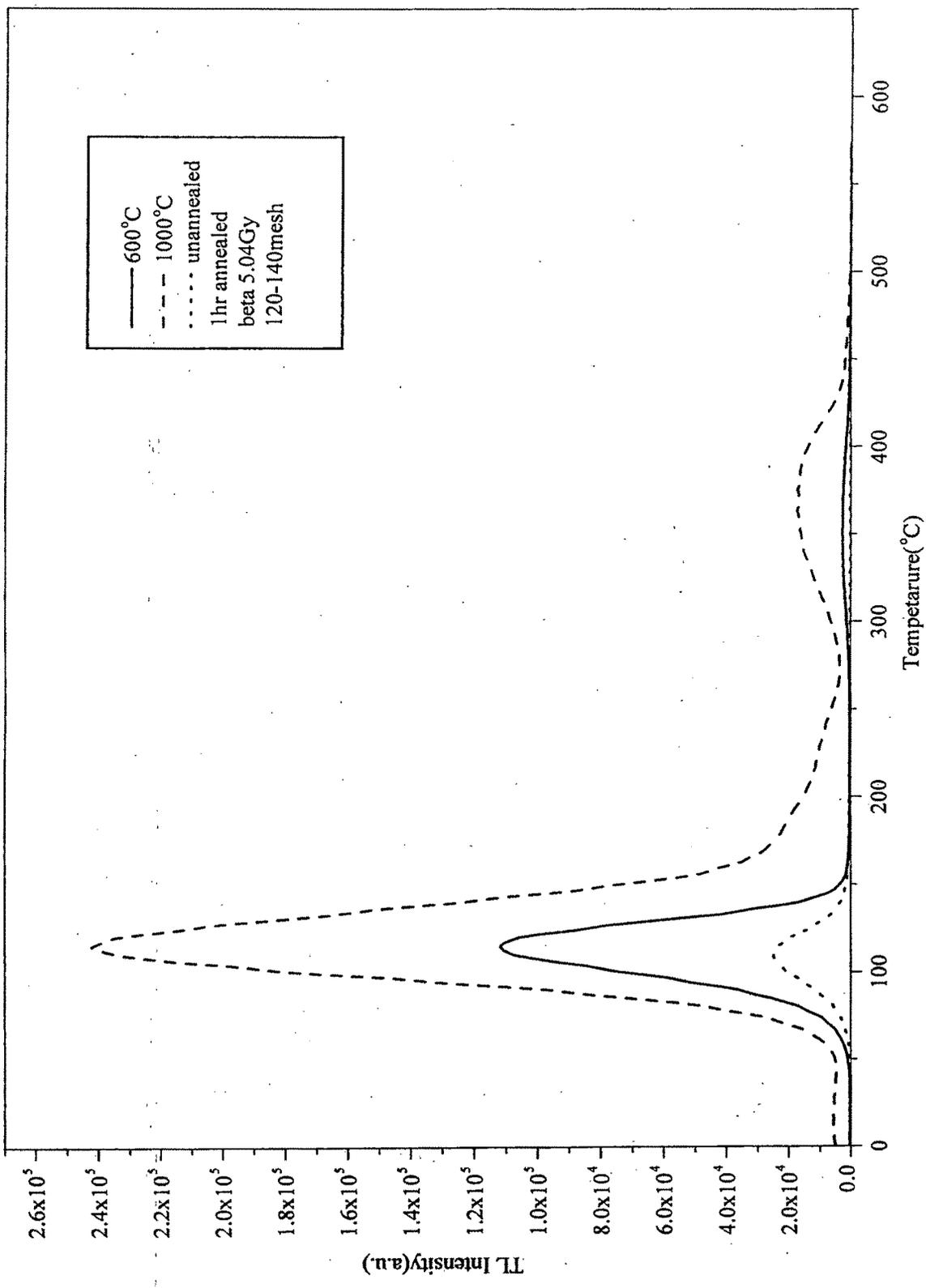
**Graph-1** TL glow curve measured at room temperature for 1hr annealed sample for a given 5.04Gy beta dose at different annealed and unannealed temperature for 120-140mesh.
