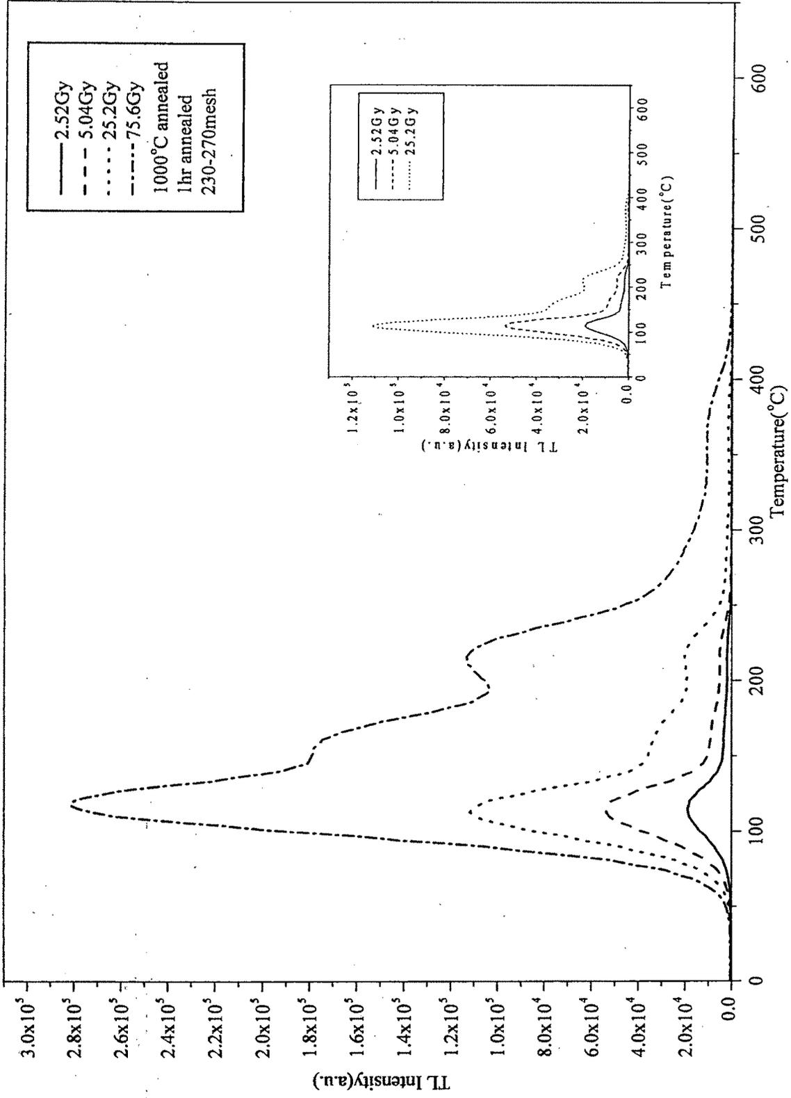
**Graph-35** TL glow curve measured at room temperature (after the OSL measured at room temperature) of 1000 °C annealed sample for 1hr duration at different doses for 230-270mesh.
