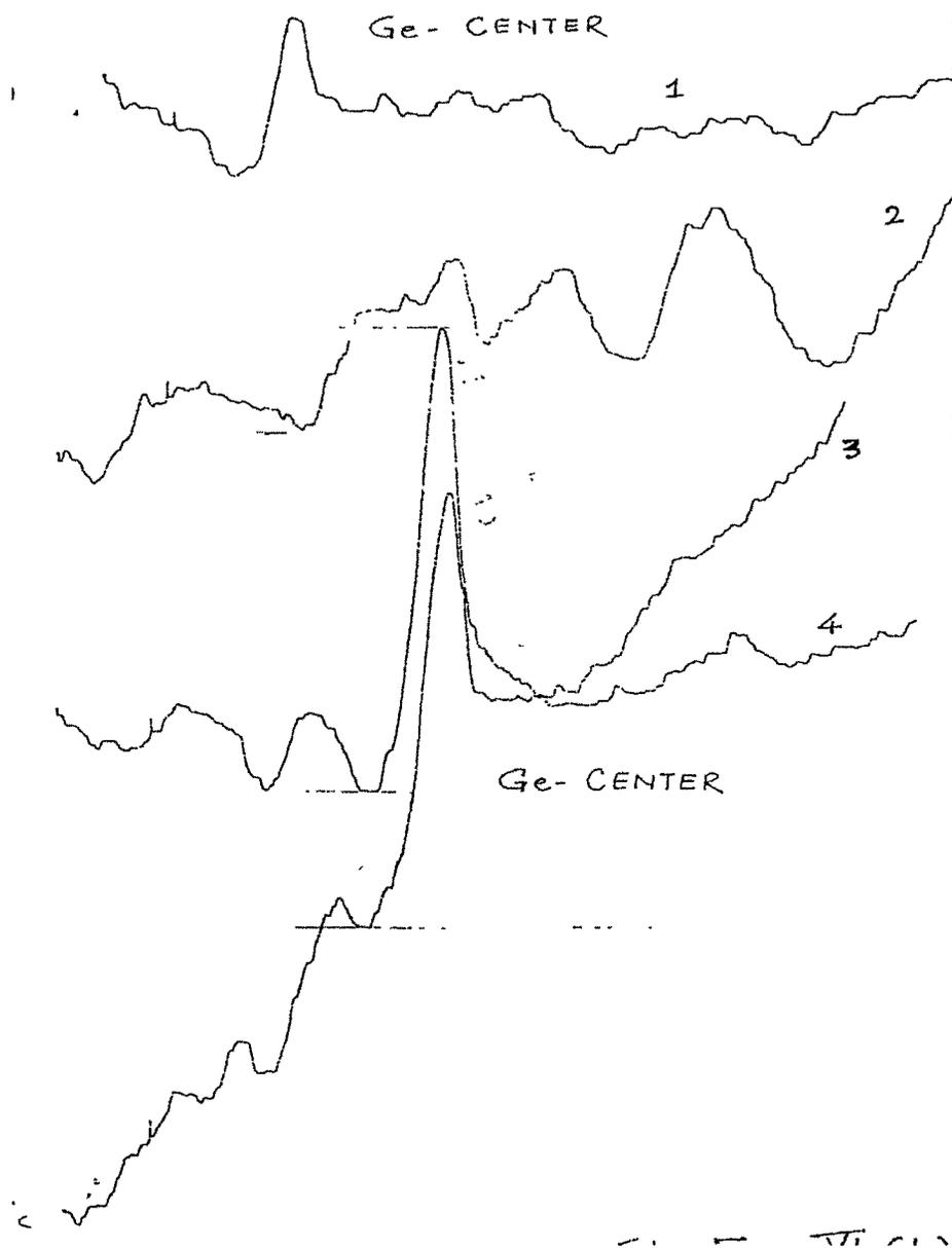
**ESR Spectra-VI(b)** ESR spectra recorded at room temperature after UV illumination for Ge Center of unannealed and annealed sample for 230-70mesh at a given gamma dose of 1000 Gy.
