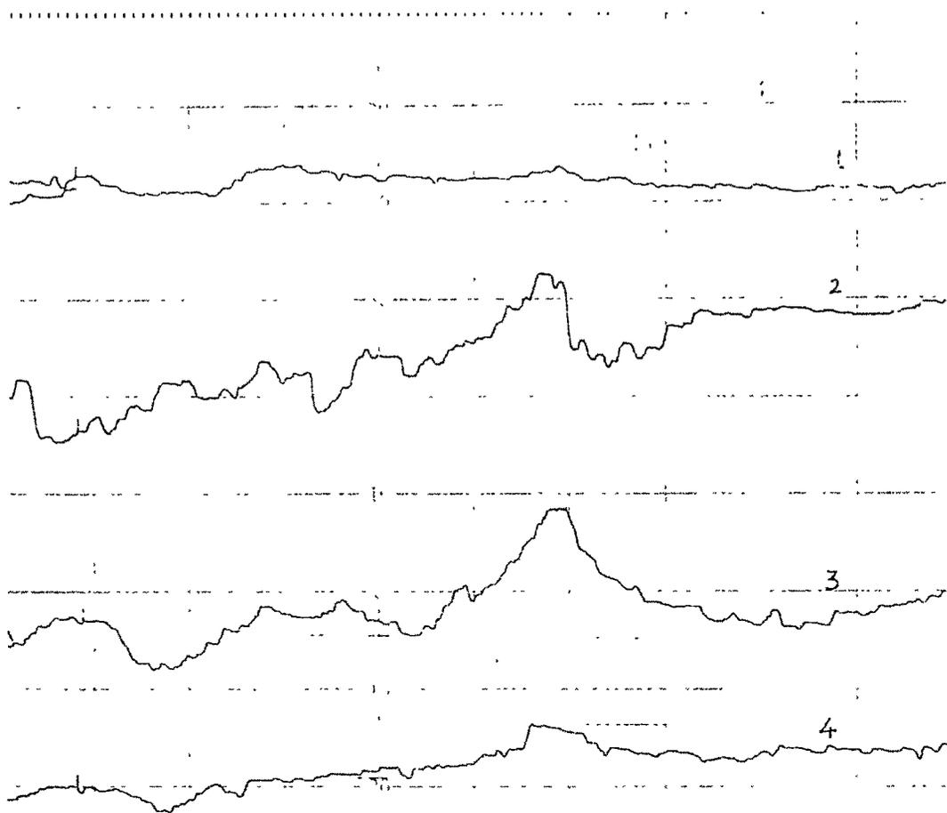
**ESR Spectra-III** ESR spectra recorded at room temperature of 400°C and 1000°C annealed sample for 230-70mesh at a given gamma dose of 600 Gy.
