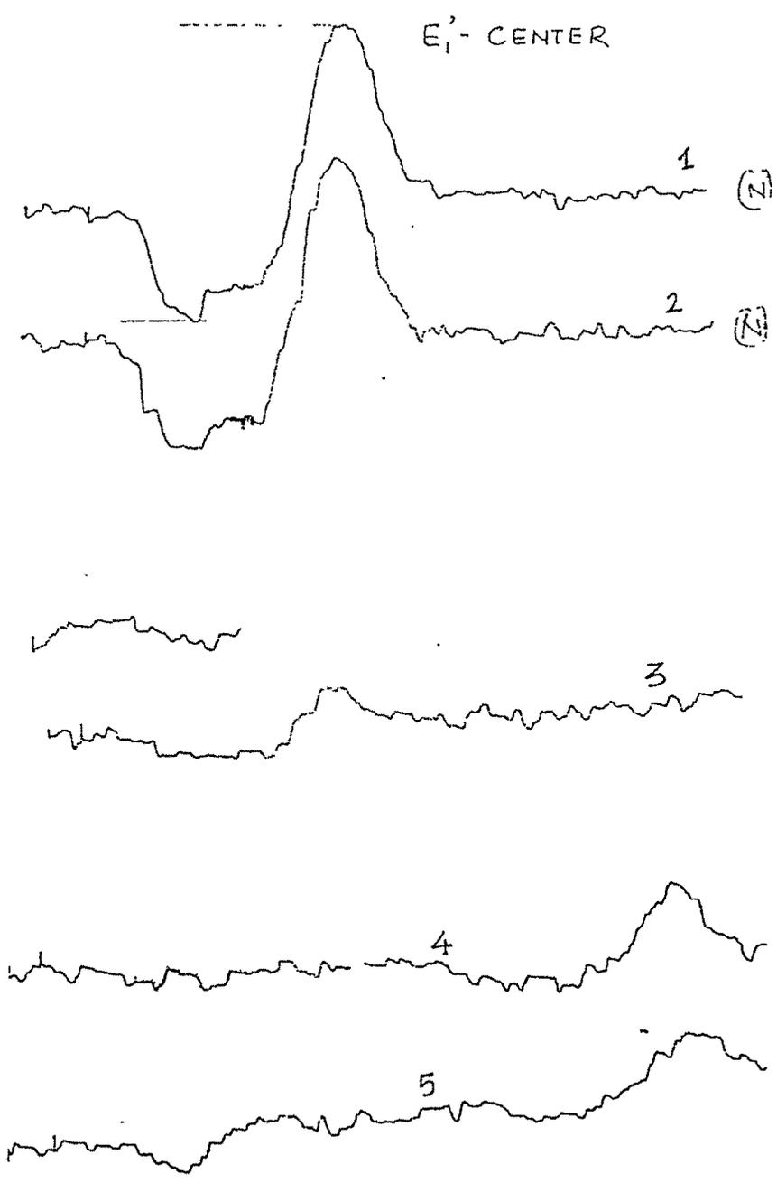
**ESR Spectra-VI(a)** ESR spectra recorded at room temperature after UV illumination for  $E_1'$  Center of unannealed and annealed sample for 230-70mesh at a given gamma dose of 1000 Gy.
