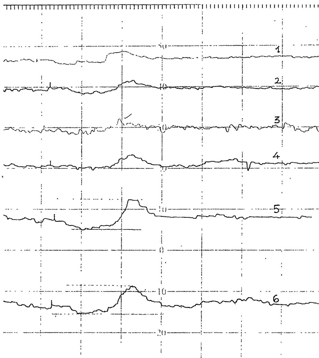
**ESR Spectra-I** ESR spectra recorded at room temperature of unannealed sample for 230-270mesh at different gamma doses.
