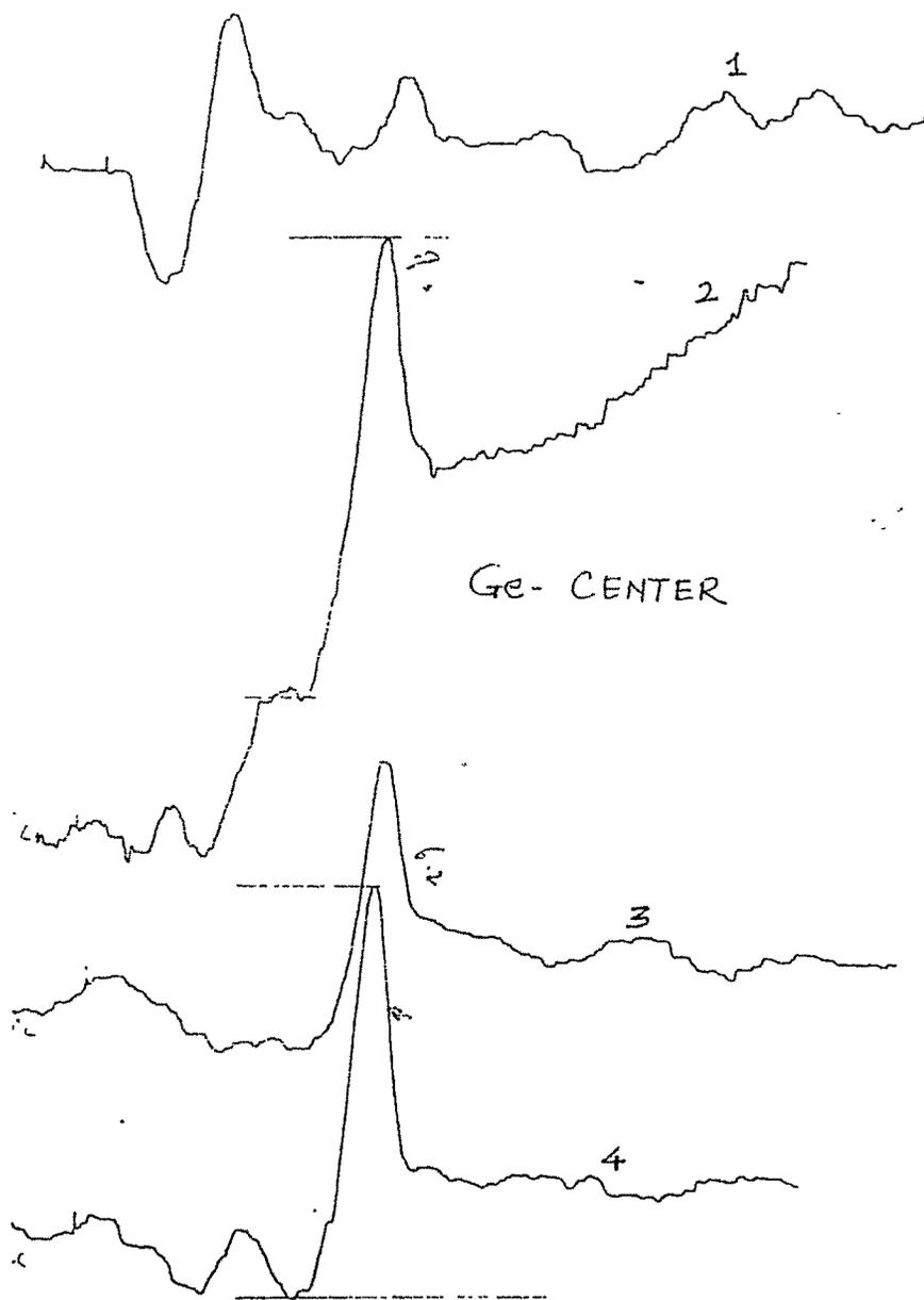
**ESR Spectra-V(b)** ESR spectra recorded at room temperature before UV illumination for Ge Center of unannealed and annealed sample for 230-70mesh at a given gamma dose of 1000 Gy.
