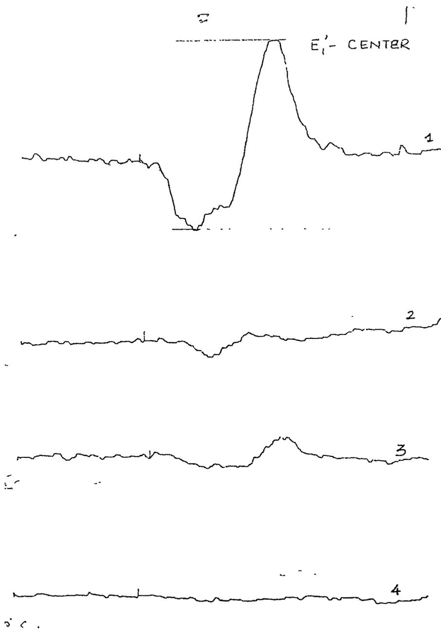
**ESR Spectra-V(a)** ESR spectra recorded at room temperature before UV illumination for E<sub>1</sub>' Center of unannealed and annealed sample for 230-70mesh at a given gamma dose of 1000 Gy.
