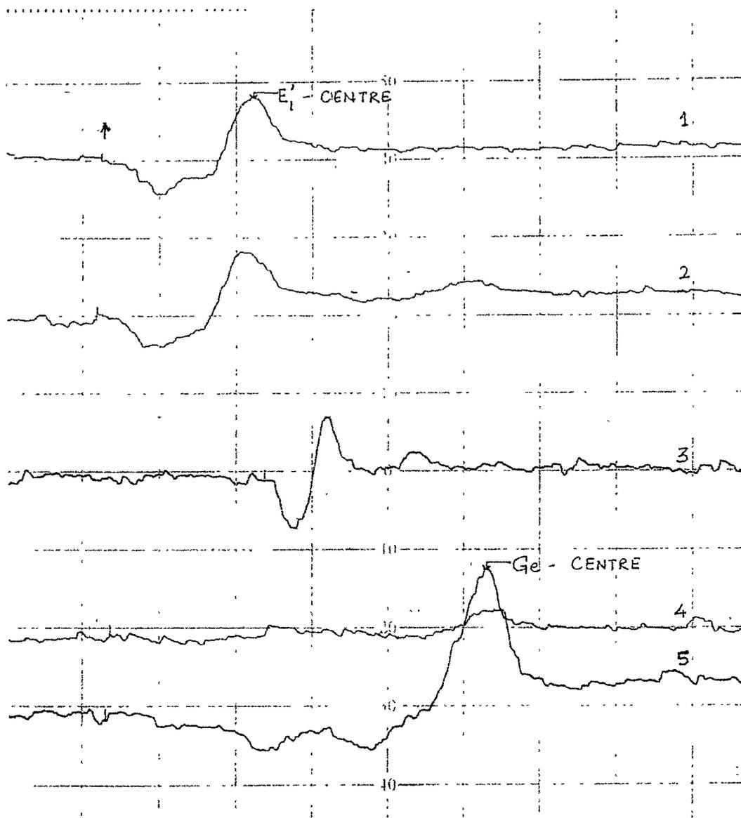
**ESR Spectra-II** ESR spectra recorded at room temperature of unannealed and 600°C sample for 230-270mesh at a constant gamma dose of 1000Gy.
