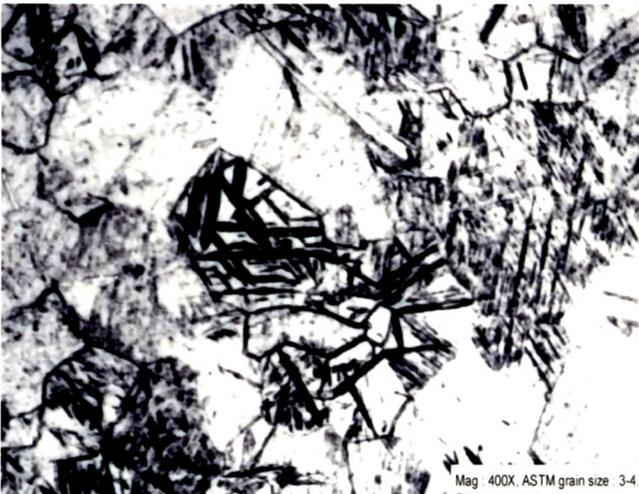
Figure - 4.3 : Photomicrograph of Normalized Titanium showing grains & hydrides of Titanium.
