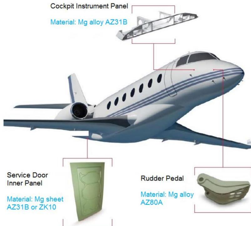
**Figure 2.14** Various parts made by Mg alloys in aeroplane [51]
