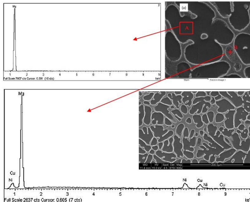
**Figure 2.22** SEM-EDS analysis of Mg-3%Ni-3.0%Cu alloy [112]
