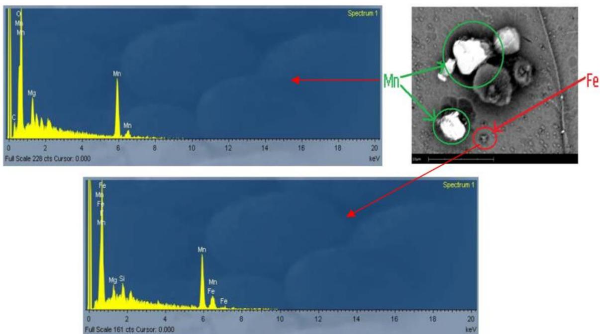
**Figure 2.20** SEM-EDS analysis 4.07 wt. %Mn and 0.061wt. %Fe [76]
