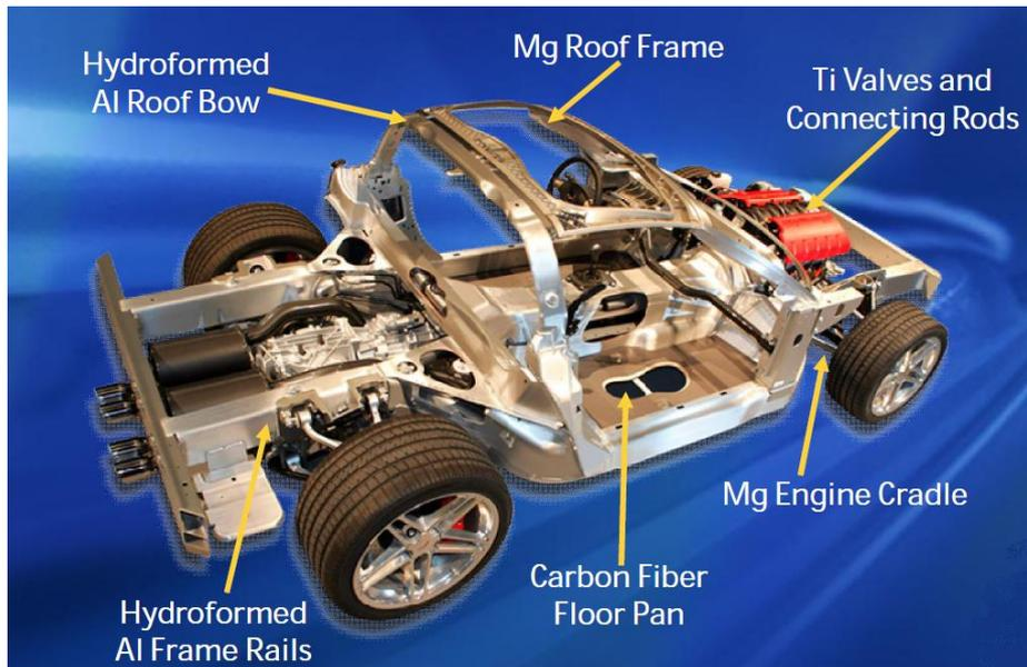
**Figure 2.12** (a) Use of Mg alloys in various automobile parts (b) GM Chevrolet Corvette Z06 [52, 54]
