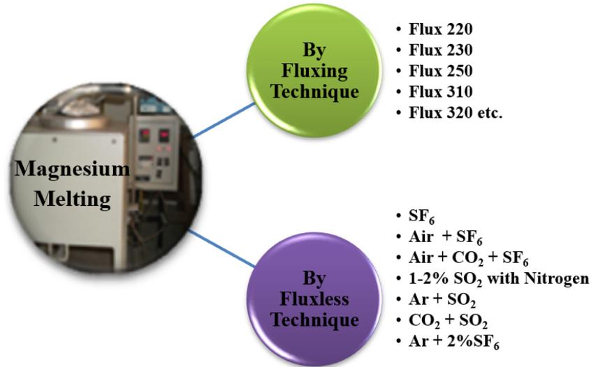
**Figure 2.23** Fluxes/Gases used during magnesium melting
