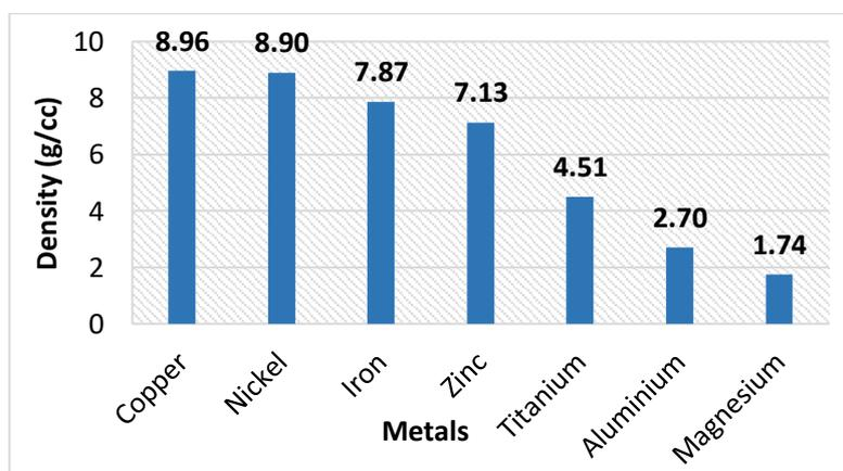
**Figure 2.1** Density of different metals (g/cc) [29]
