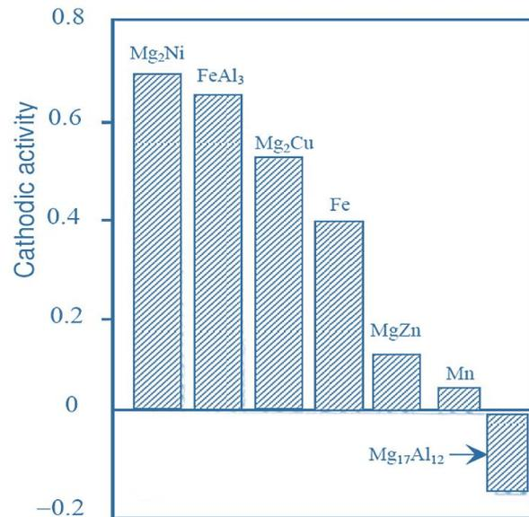
**Figure 2.21** Compared to their alloy matrix, the cathodic activity of precipitated phases of Mg alloys in salt water [95]
