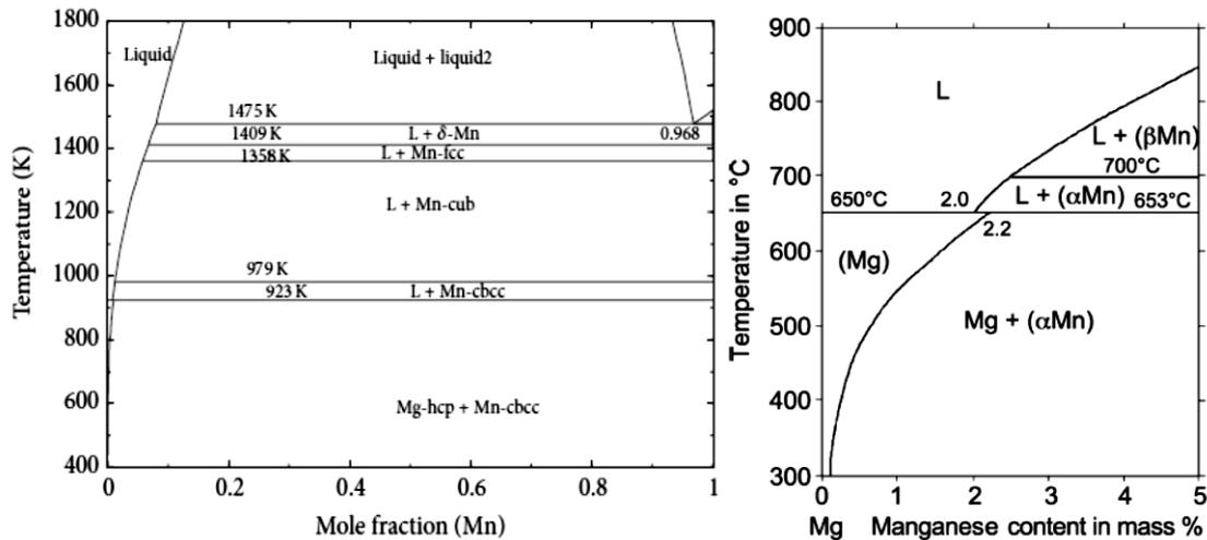
**Figure 2.19** Mg-Mn binary phase diagram [10, 34, 66]
