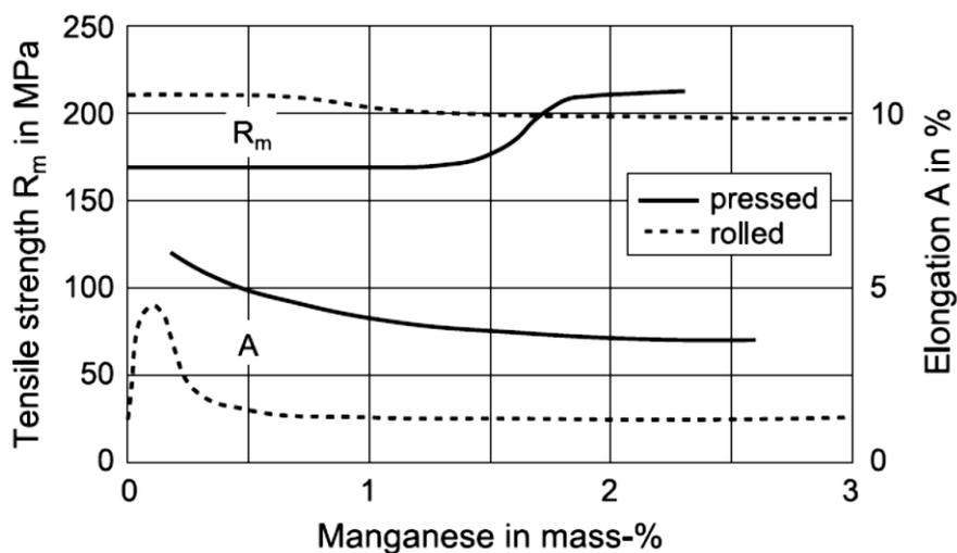
**Figure 2.18** Effect of Mn on the mechanical properties of magnesium [34]
