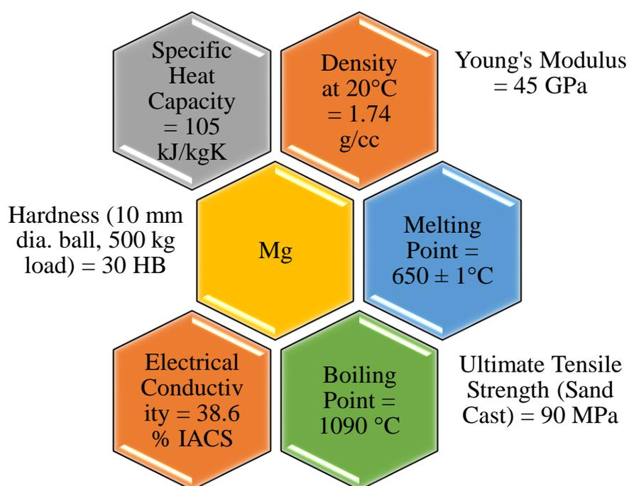
**Figure 2.5** Some physical, electrical, and mechanical properties of magnesium [26, 28]
