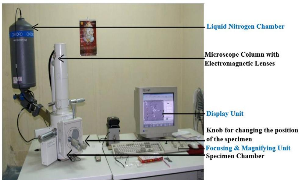
**Figure 3.13** Scanning Electron Microscope (JEOL JSM-5610LV) with EDS
