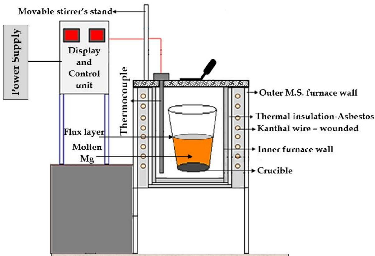
**Figure 3.2** Schematic diagram of experimental setup
