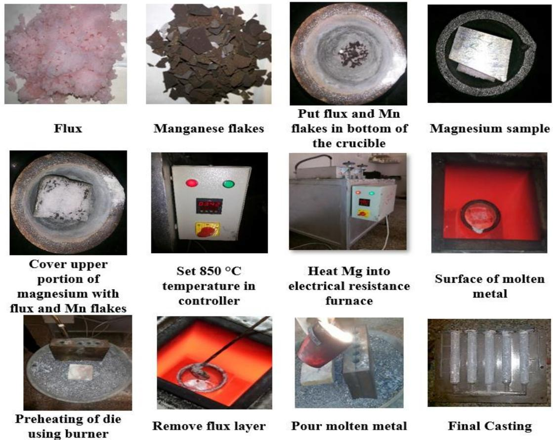
Figure 3.7 Experimental steps of Mg-Mn flakes system
