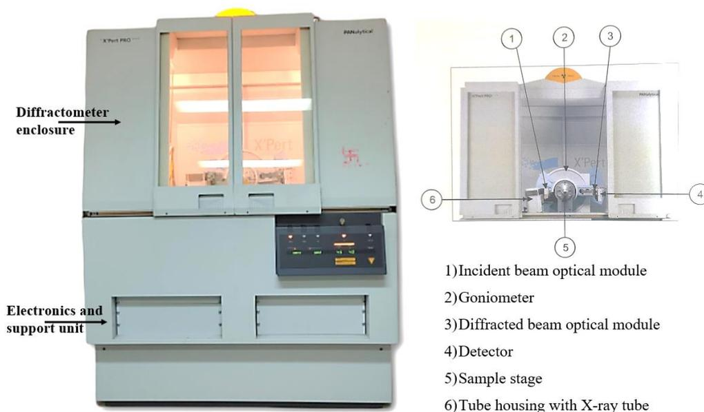
**Figure 3.14** X-ray diffraction system
