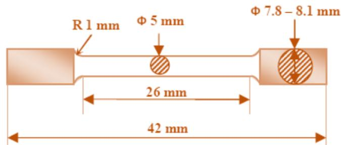
**Figure 3.16** Line diagram of tensile test specimen
