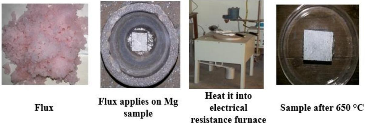
**Figure 3.5** Steps for surface layer of flux on magnesium
