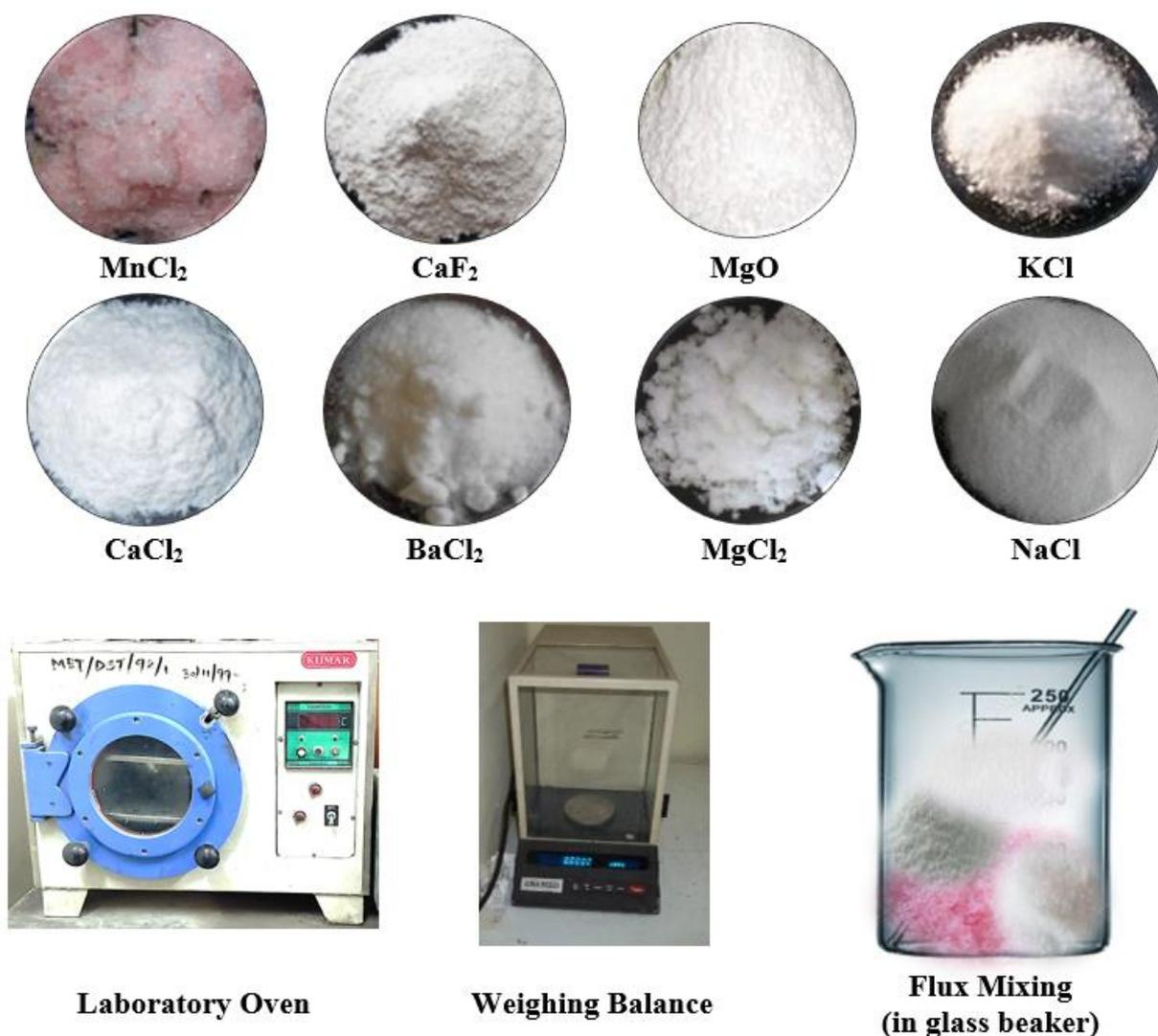
**Figure 3.4** Chemicals, Equipments and apparatus used in flux preparation
