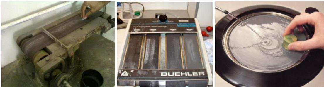
**Figure 3.11** Grinding and Polishing steps
