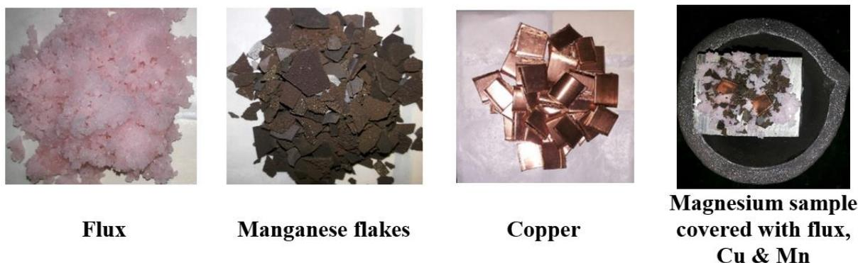
**Figure 3.8** Materials used to develop Mg-Cu and Mg-Cu-Mn alloys
