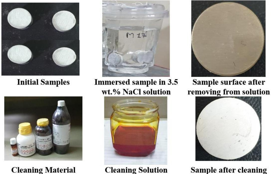
**Figure 3.19** Immersion test samples and materials
