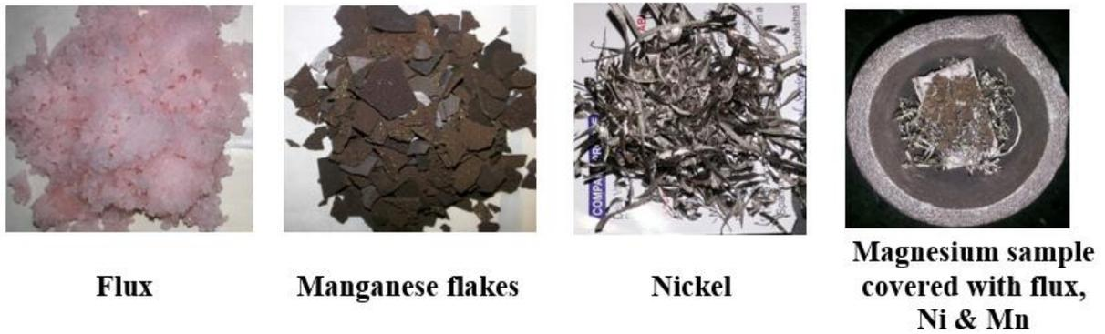
**Figure 3.9** Materials used to develop Mg-Ni and Mg-Ni-Mn alloys
