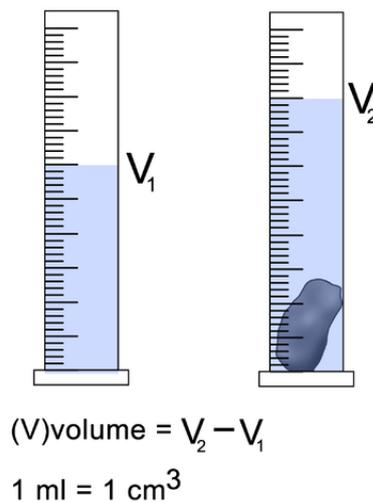
**Figure 3.18** Density measurements by water displacement method
