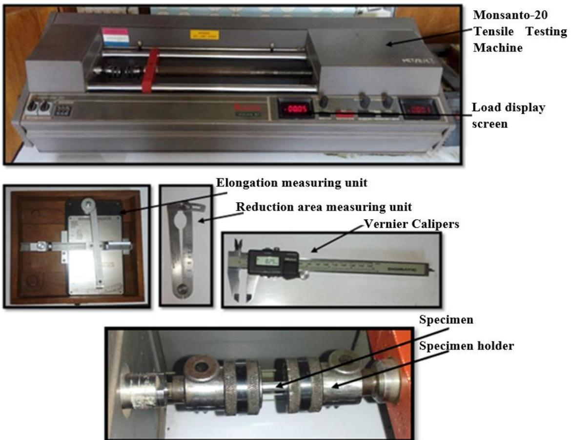
**Figure 3.17** Monsanto-20 tensile testing equipment & its related accessories
