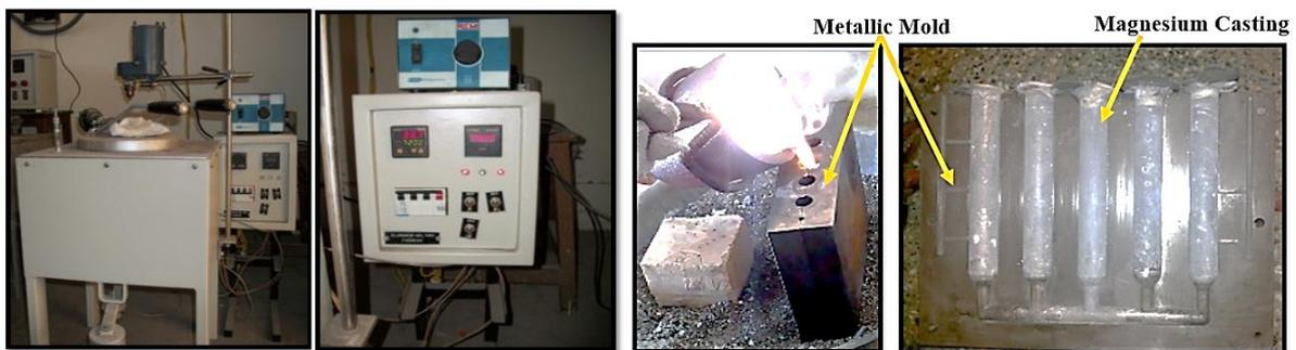
**Figure 3.6** Experimental setup and final casting
