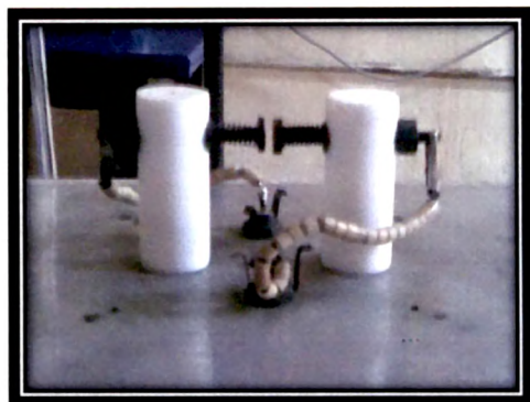
Fig.3.3. Sample holder for the conductivity measurement.
