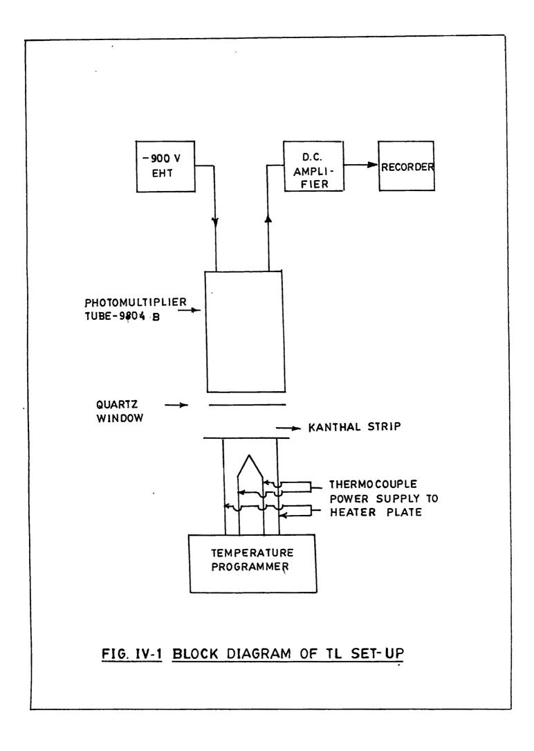
The TL glow curve recorder system consists of a photomultiplier tube, a high voltage DC supply unit, a DC amplifier, a temperature programmer and X-Y strip chart recorder. Block diagram of the unit is shown in Fig.IV-1.
