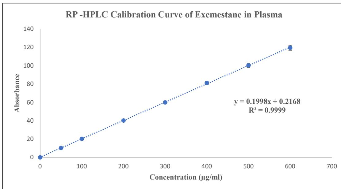
Figure 4.25 Calibration plot of Exemestane by RP – HPLC in rat plasma
