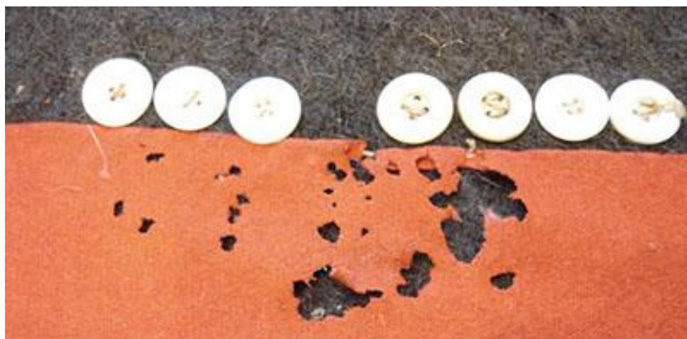
Fig 2.4: Irregular shaped holes in wool fabric caused by insect attack
