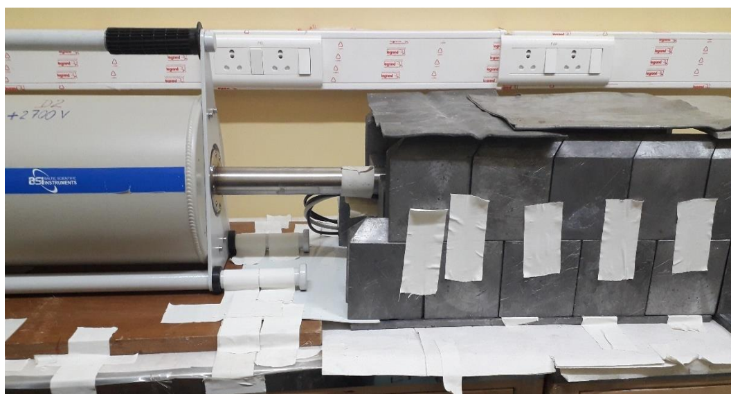
Fig. 2.7 Off-line \gamma -ray spectrometry method setup along with lead shield HPGe detector.
