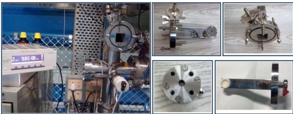
Fig. 2.2 The 6M irradiation set-up and target assemblies at BARC-TIFR Pelletron accelerator facility Mumbai.
