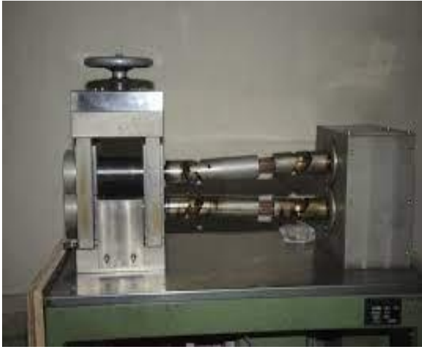
Fig. 2.3 Sample preparation rolling machine and pelletizer at target lab of BARC-TIFR facility.
