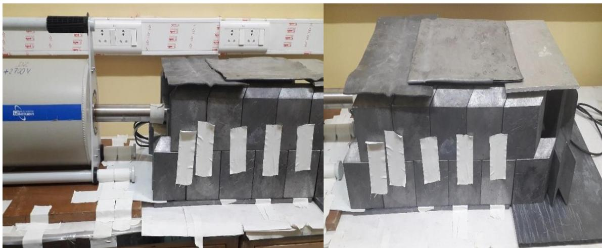
*Fig. 3.4 The HPGe detector which is properly shielded by lead reduces the contribution of natural radioactivity.*
