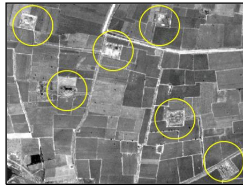
Identification of oil well from Cartosat-1 satellite image
