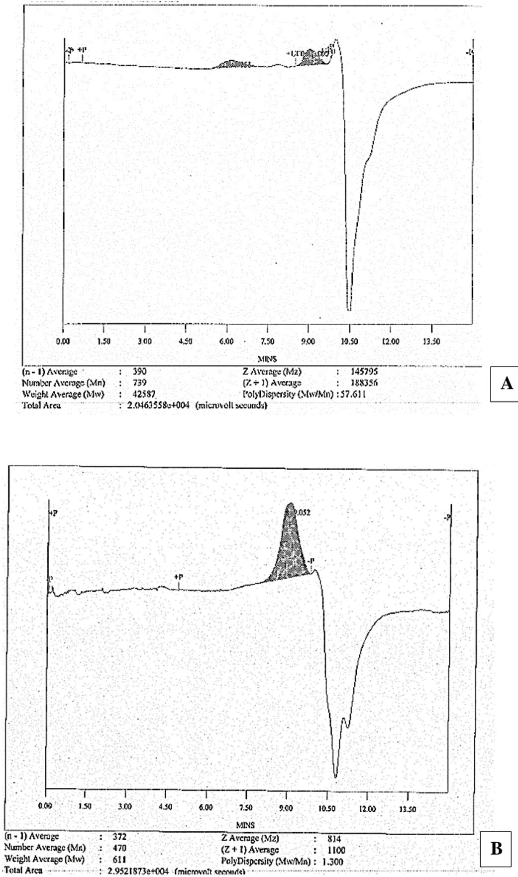
Figure.52. Gel-permeation chromatography analysis: A- Untreated PE film; B- Nitric acid pre-treated PE film
