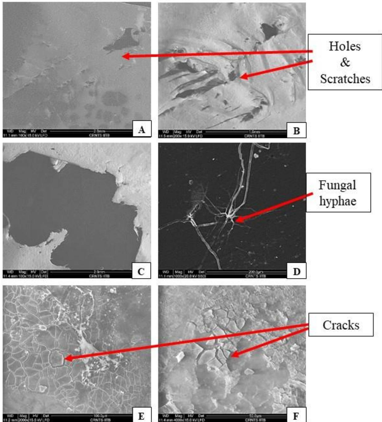
**Figure.50. A- Experimented film after 10- & 20-day incubation displaying fungal hyphae penetration, hole and cracks: A & B- Holes and scratches after 10-day incubation (100x, 200x); C- Hole after 20-day incubation (200x); D- Fungal hyphae penetration and cracks on the surface after 10-day incubation(1000x); E- Torn film developing a big hole after 20-day incubation (200x); E, F- Cracks on the surface of experimented PE film (2000x, 4000x)**
