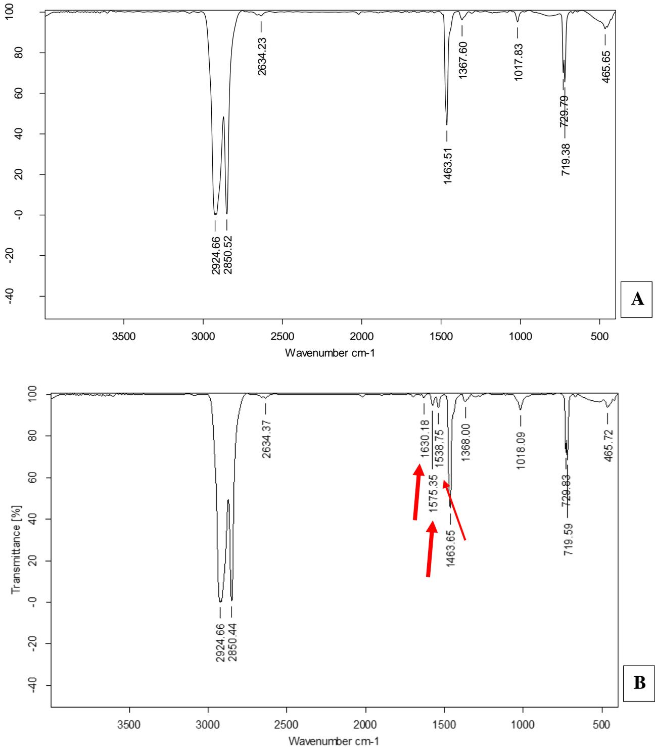
**Figure.47. FTIR spectra of experimented PE films in lab-simulated area at optimum conditions: A- Pre-treated film; B- Experimented PE film with maximum weight-loss (arrow-formation of new peaks)**
