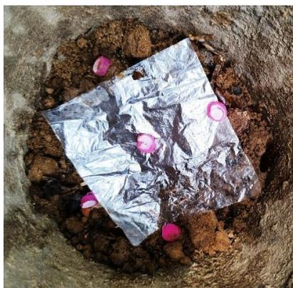
**Figure.43. Arrangement of the fungal inoculum & film in soil and mulch medium (Experimental medium)**
