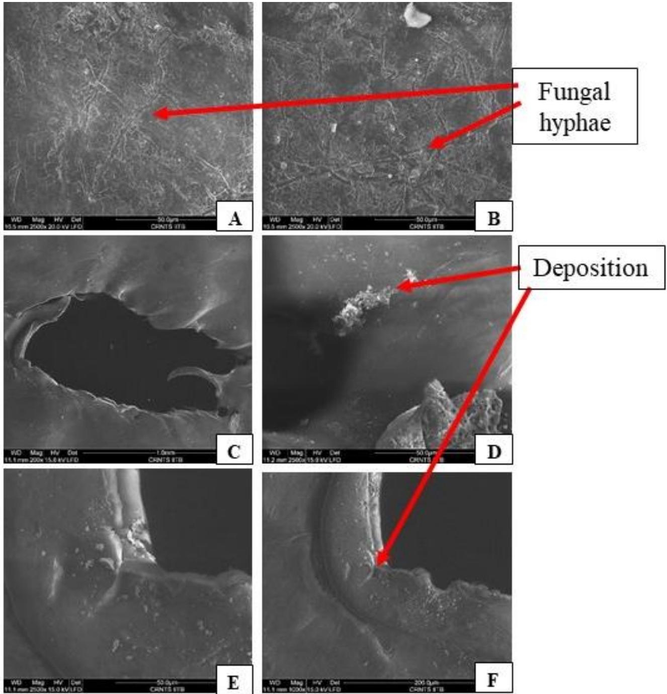
**Figure.46. A- Experimented film after 10- & 20-day incubation displaying fungal hyphae penetration, hole and polymer fragments: A & B- Fungal hyphae penetration and cracks on the surface after 10-day incubation(2500x); C- Torn film developing a big hole after 20-day incubation (200x); D, E, F- Magnified images of a hole showing fragmented polymer in the margin (2500x, 2500x, 1000x)**
