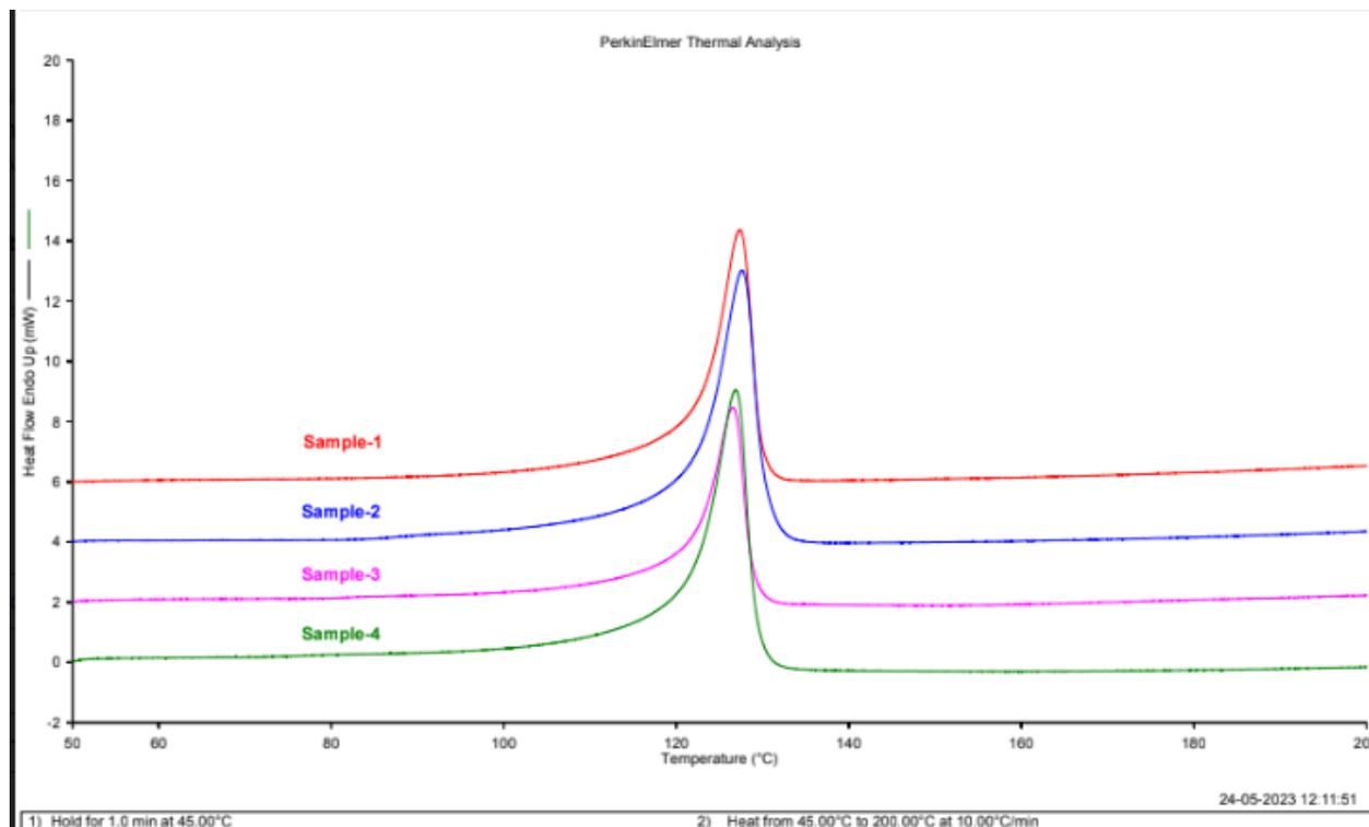
**Figure.54.** An overlay thermogram of Differential Scanning calorimetry (DSC) analysis performed on experimented films: **Sampe 1-** Untreated PE film; **Sample 2-** Pretreated film without fungal treatment; **Sample 3-** Pretreated film experimented with SA17 with tween 80 supplementation; **Sample 4-** Pretreated film experimented with SA17 without tween 80 supplementation
