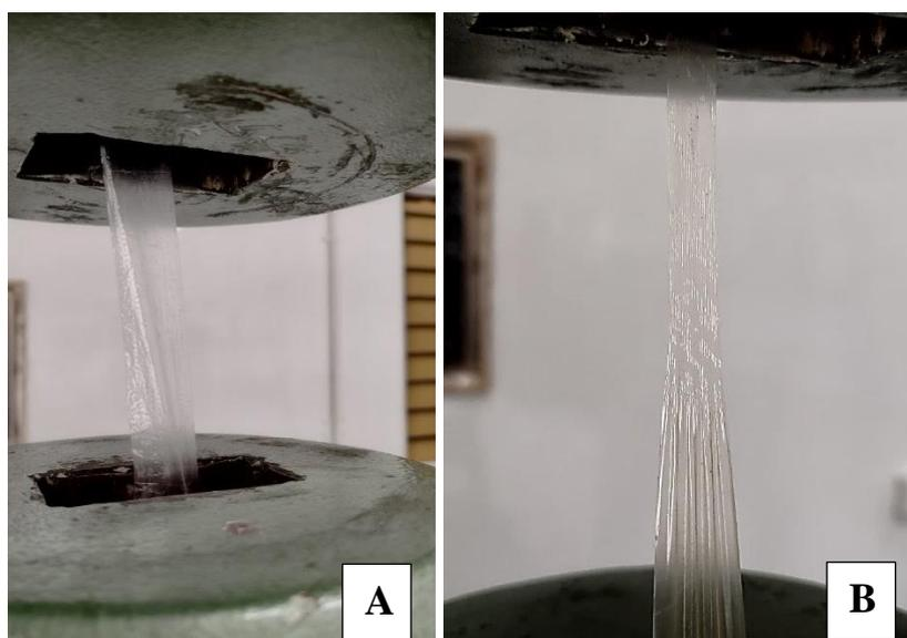
**Figure.55. Tensile strength analysis of the experimented PE films: A-PE film at the starting point; B- PE film right before the ending point**
