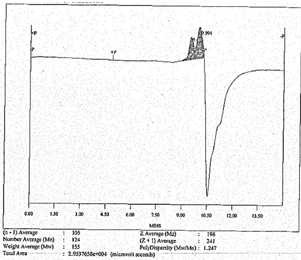
**Figure.53. Gel-permeation chromatography analysis:** Fungal treated PE film at optimum conditions
