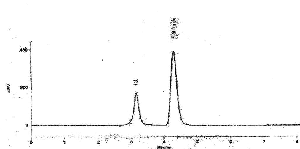
According to the conditions described, the retention times for FLT were about 4.02 min and 5.1 min for IS and FLT in rat plasma, respectively. Typical chromatograms of blank rat plasma, plasma with IS, plasma with IS and FLT are shown in Fig. 4.2 to 4.4.
