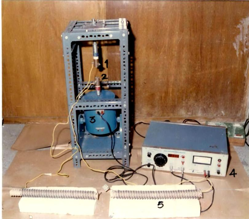
**Fig. 3.10 :** Photograph of the contact testing set-up for a pair of contacts.
