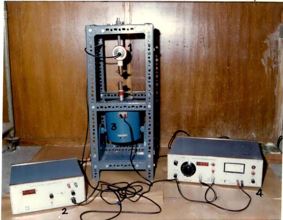
**Fig. 3.9 : Photograph of the contact force measurement set-up**
