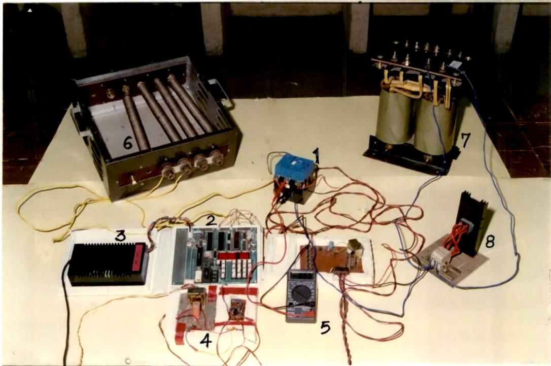
**Fig. 3.17 : Photograph of the DC contact testing set-up**
