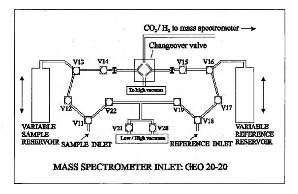
Fig 2.2. Schematic diagram of  $CO_2$  preparation using CAPS and the Mass Spectrometer inlet system.
