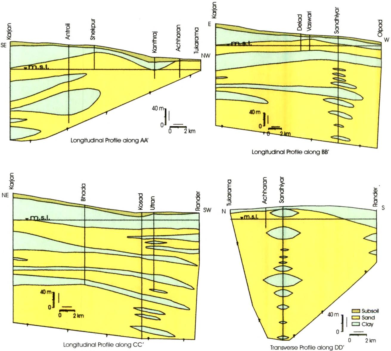
**Fig. 3.7 - Diagram Showing The Sub-Surface Transverse (D - D') And Longitudinal (A - A', B - B' And C - C') Profiles Along Tapi Lobe - II.**
