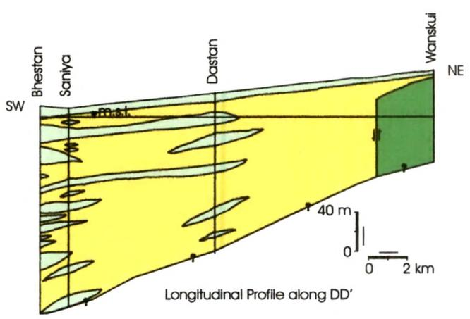
**Fig. 3.5 - Diagram Showing The Sub-Surface Transverse (A - A') And Longitudinal (B - B', C - C' And D - D') Profiles Along Tapi Lobe - I.**
