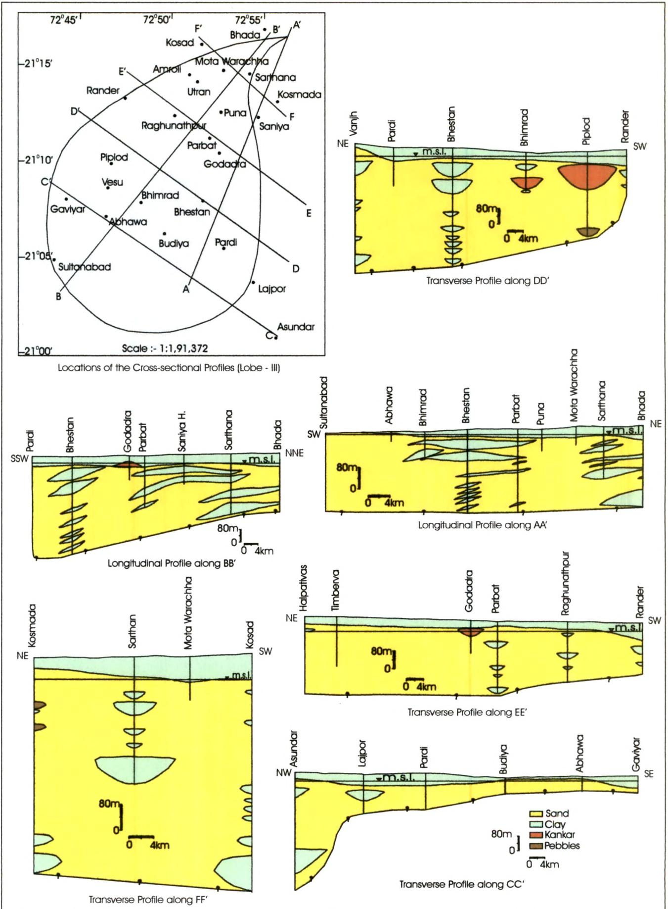
**Fig. 3.9 - Diagram Showing The Sub-Surface Transverse (C - C', D - D', E - E' And F - F') And Longitudinal (A - A' And B - B') Profiles Along Tapi Lobe - III.**
