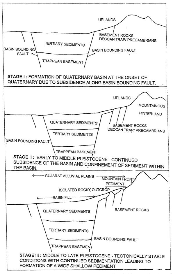
Fig. 8.2 Idealised E-W cross-sections across Gujarat alluvial plains showing stages in Quaternary basin evolution.
