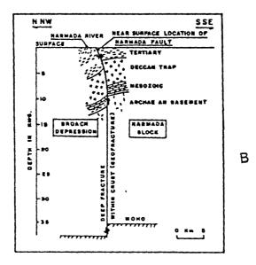
Fig. 8.5 A - Seismic section of southern Cambay basin and B - Cross section across Narmada geofracture showing nature of Narmada fault (after Roy, 1991).
