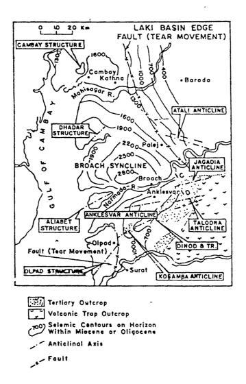
Fig. 8.3 Quaternary subsurface folds and faults in southern Cambay basin (after Sudhakar et al., 1970).
